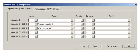
In the register "Logic definitions" you link the connections with the requested events.
