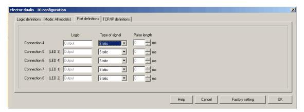
The field "Logic" shows the basic function of the pin. In the selection field "Type of signal" you set whether this is a static signal or signal pulse (pulse). In the event of a signal pulse, you can define the requested pulse length from 50...1000 ms in the following input field.
