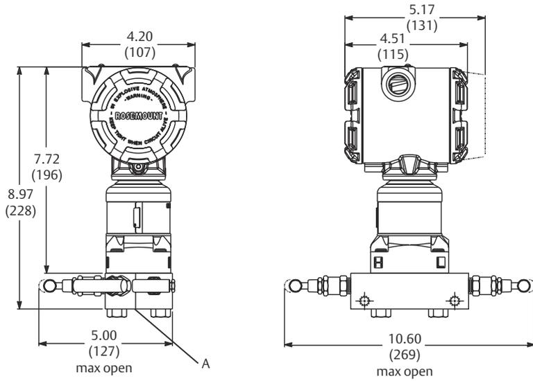
A. 1/2-14 NPT on manifold for process connections, 2 1/8-in. (53.98 mm) center-to-center, 1/4-18 NPT for test/vent connection
