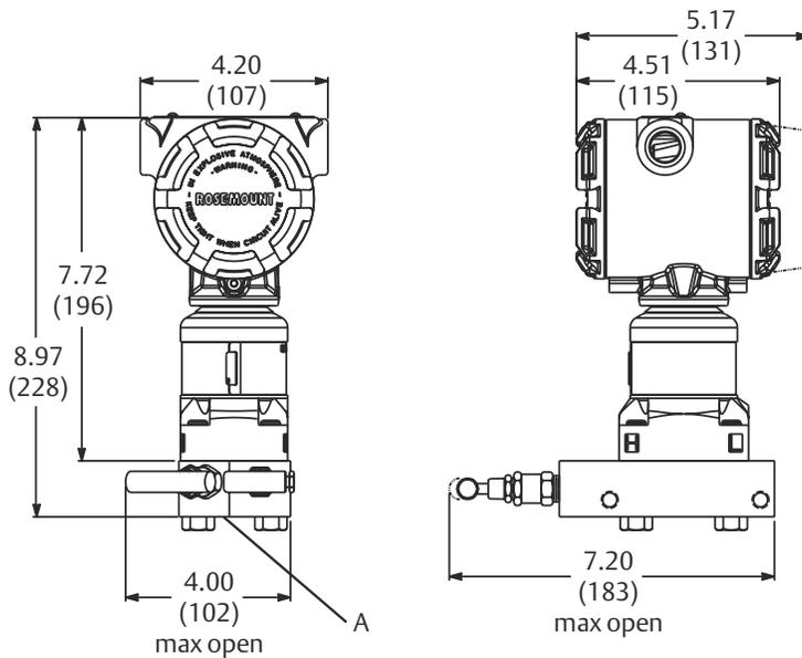
A.  $\frac{1}{2}$ -14 NPT on manifold for process connection,  $\frac{1}{4}$ -18 NPT for test/vent connection
