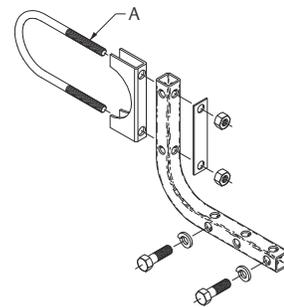
A. 2-in. (50.8mm) U-bolt for pipe mounting
