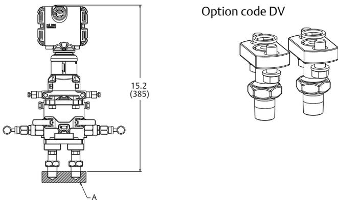
A. Cross section image is shown for dimensioning purposes only; it is not part of the transmitter assembly
