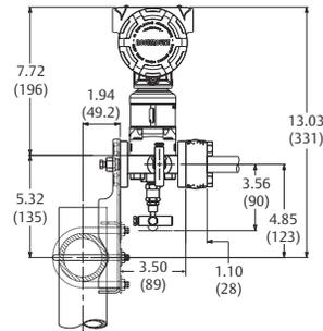
Manifold handle assembly may vary slightly from image shown. All valve handle assemblies provide the same function and meet all stated drawing dimensions.
