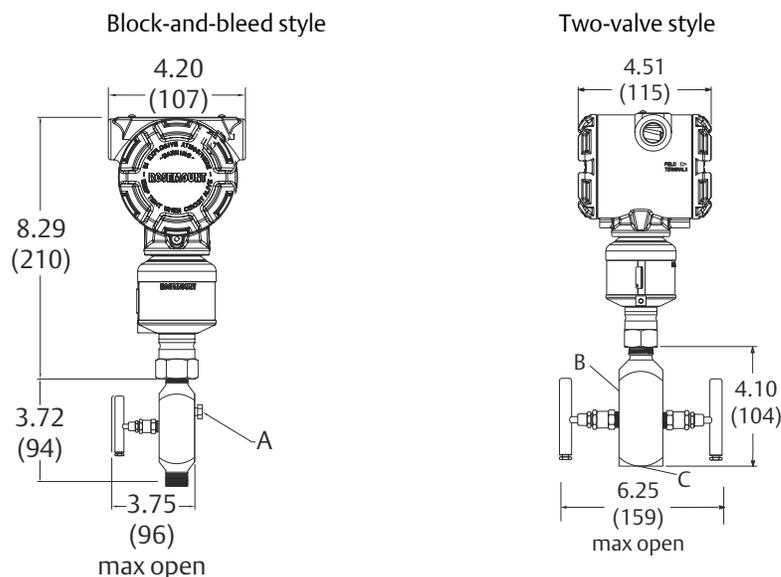
A. Bleed screw (unspecified dimension)- not C.  $\frac{1}{2}$ -14 NPT female NPT process connection (code BA) designed for accessory attachments
