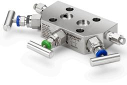
Rosemount Coplanar manifolds provide a leak checked and pressure tested single point solution when assembled to Rosemount pressure transmitters. The coplanar platform reduces potential leak paths by 50 percent over conventional style process connections while also reducing overall connection system weight.
