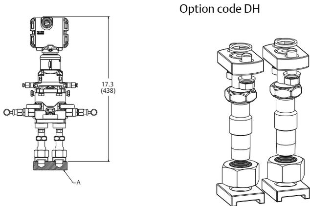
A. Cross section image is shown for dimensioning purposes only; it is not part of the transmitter assembly
