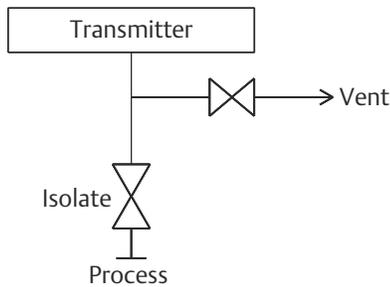
**Figure 3: Rosemount 304 Manifold**
