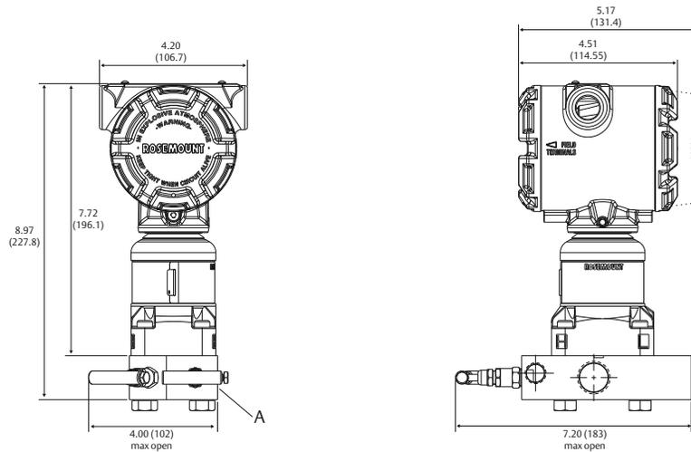
A. 1/2-14 NPT on manifold for process connections, 1/4-18 NPT for test/vent connection
