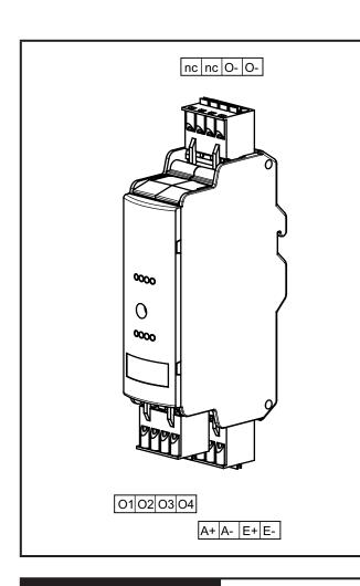
O-: switching output actuator 0 V
