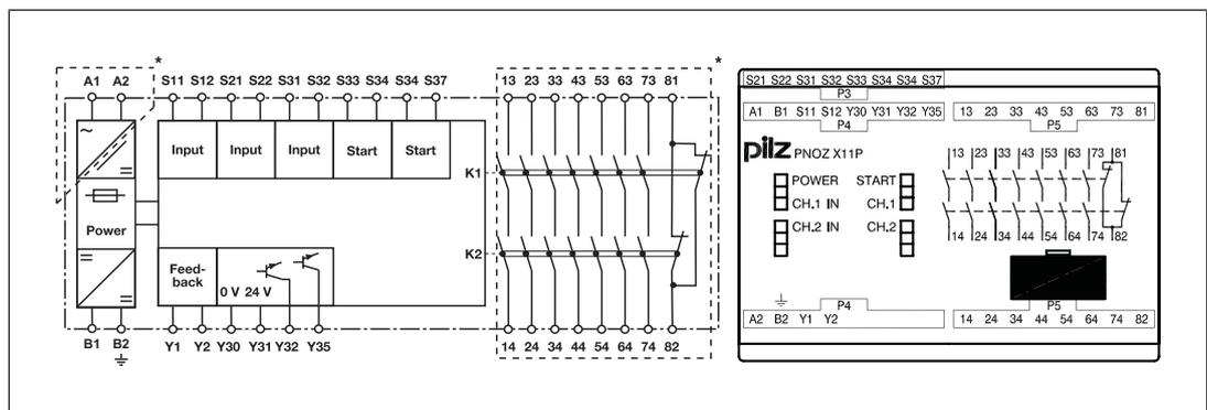
\*Insulation between the non-marked area and the relay contacts: Basic insulation (over-voltage category III), Protective separation (overvoltage category II)
