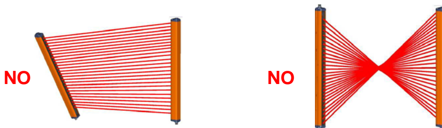
Fig. 14 – Light curtain alignment
