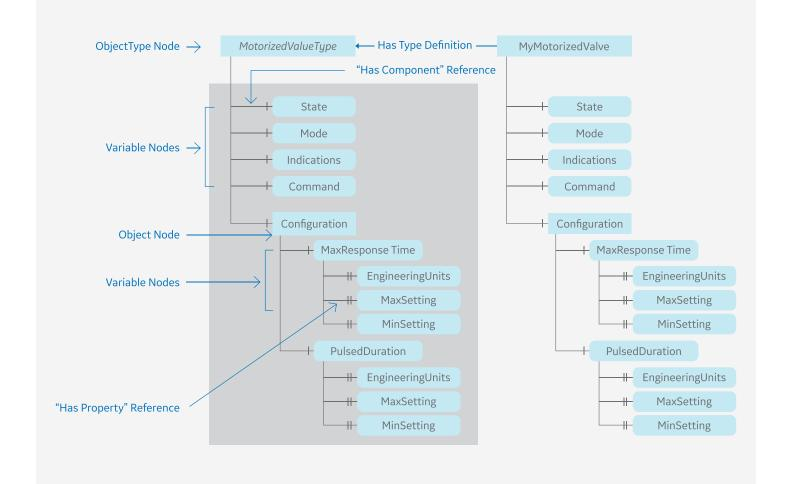
Figure 5 - OPC ObjectType Definition for a Motorized Operated Valve
