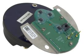
4. Attach the removed EB board to the new Modbus terminal block.
