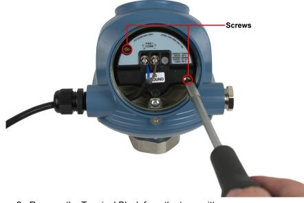
2. Remove the Terminal Block from the transmitter.
