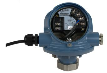
2. Attach the communication cables to the new terminal block.
