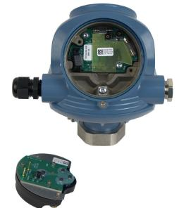
3. Detach the EB board by pulling it straight out from the backside of the existing terminal block.
