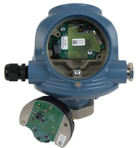
5. Attach the IS Ground Label to the front of the terminal block.
