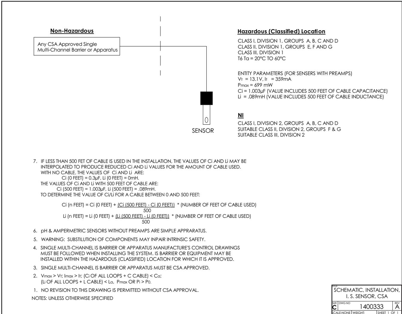
The pH sensors listed below can be used with this installation drawing. Sensors may or may not contain an integral preamplifier.
