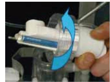
12. Connect the VP cable to the sensor. The sensor connector is keyed to ensure proper mating with the cable receptacle. Once the key has slid into the mating slot, hand tighten the connection by turning the knurled ring clockwise.
