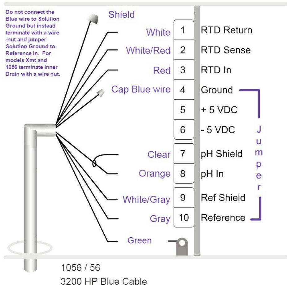
Figure 3-2: Rosemount 3200HP Sensor Wiring to Rosemount 1057 Transmitter
