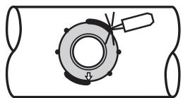
► Apply the welding seams between the fixing points opposite each other. Ensure sufficient intervals between the individual sections (cooling phases to avoid glowing through / warping of the adapter due to overheating).
