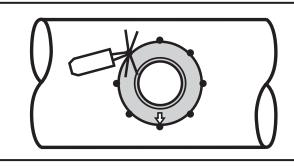
► Fix the adapter in several spots with a sufficient adhesive force; apply the fixing points at equal distance opposite each other.
