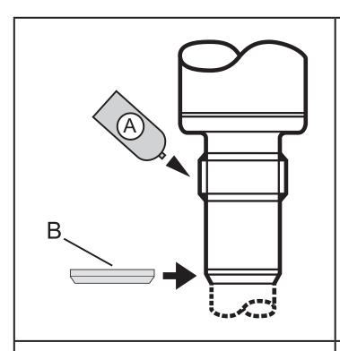
► Lightly grease the thread of the sensor using a lubricating paste (A).
