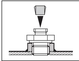
4. Attach the coupling nut and insert the sensor (D).
