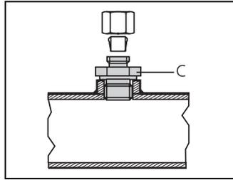
2. Grease all parts of the adapter: coupling nut (A), progressive ring (B), thread and cone of the fitting (C).
