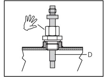
5. Tighten the coupling nut manually and mark its position with a line (E).
