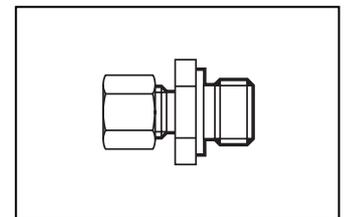
1. Insert the fitting (C) into the process connection and tighten.
