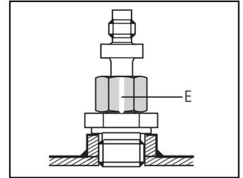
6. Adjust the sensor to the required installation depth. Hold it and tighten the coupling nut by 2 full turns.
