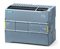
SIMATIC S7-1200F, CPU 1215 FC, compact CPU, DC/DC/DC, 2 PROFINET ports, onboard I/O: 14 DI 24 V DC; 10 DO 24 V DC; 0.5A; 2 AI 0-10 V DC, 2 AO 0-20 mA DC, Power supply: DC 20.4-28.8V DC, Program/data memory 150 KB
