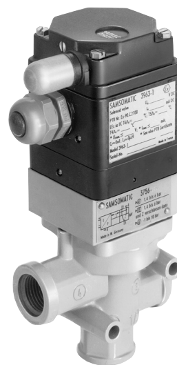
Fig. 2: 3/2-way solenoid valve · Actuated on one side · With spring return mechanism · K_{VS} 4.3 · G \frac{1}{2} connection
