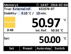
When the calibrator is stable the display will show a green  $\sum_{700}$  checkmark symbol and the instrument will emit an audible alarm. The instrument will indicate in minutes and seconds for how long the instrument has been stable.
