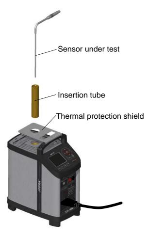
Check that the insulation plug fits the diameter of the sensor. Otherwise replace it (CTC-155/CTC-1205 only).
