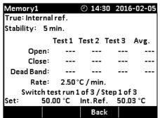
5) When dead band is not selected (single temperature change) (the graphic indicates the choice), the finished switch test result is displayed.
