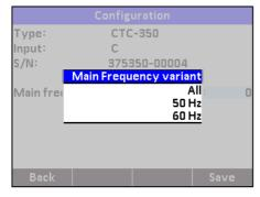
**4.** Press **F4** (Save) to save the configuration set up.
