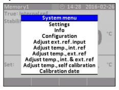
From the Maintenance System menu you can access the System Settings, the System Info, the Configuration and the Calibration date. You are also presented to a selection of adjustment options.
