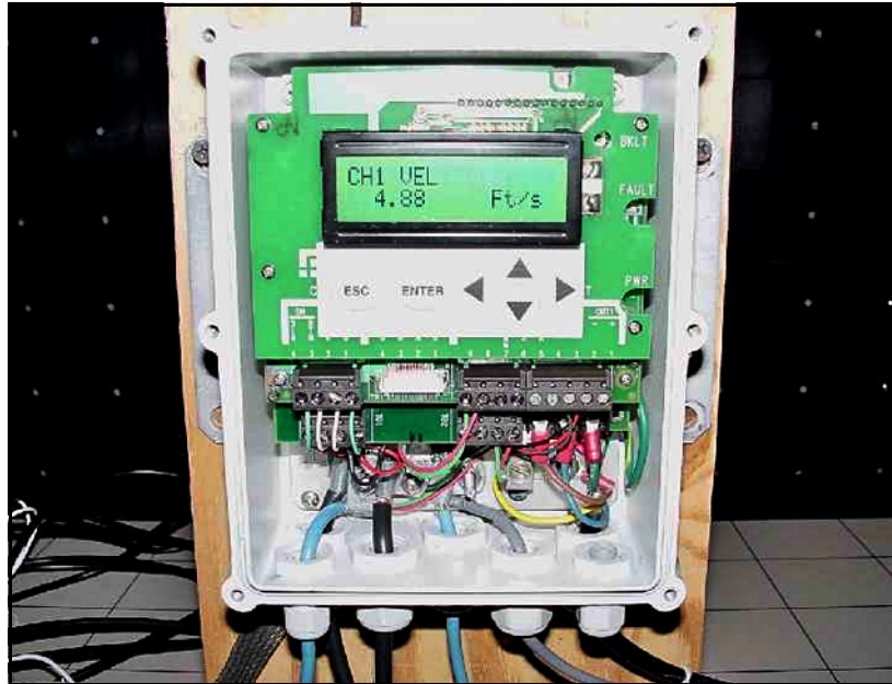
Figure 13: AT868 Properly Wired for CE Mark Compliance
