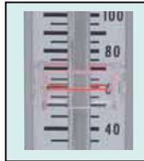
**Adjustable pointer flags** – Red lined pointer flags provide quick visual reference to a required flow level. Of clear plastic, they snap into place inside bezel and slide to desired level.
