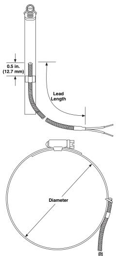
The stainless steel clamp allows temperature measurement without drilling or tapping. Ideal for measuring pipe temperatures.
