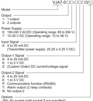
/SN: No socket (with socket if not specified) /C0: HumiSeal coating\*
