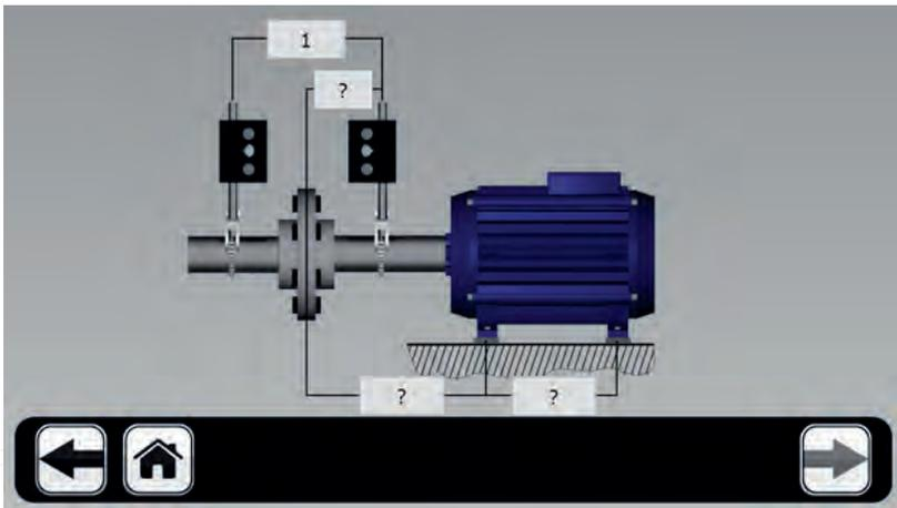
Set the units to the 12 o'clock (the green LED indicator of M and S units will glow green).
