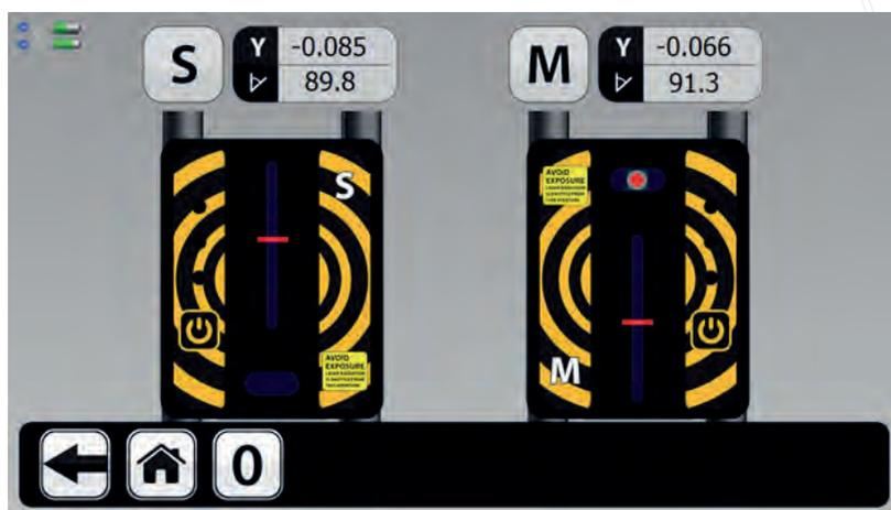
During the program loading the display shows data received directly from the sensor units (position of the laser beam on the sensor and inclinometer angle).
