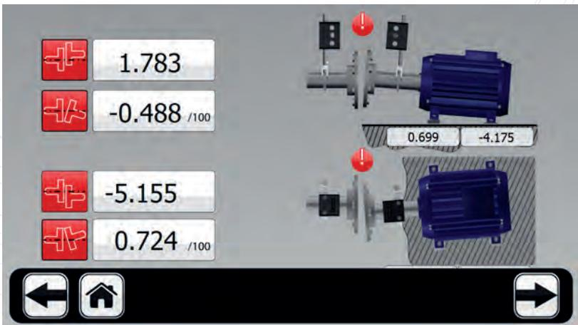
This screen shows the misalignment values according to the coupling joint and the feet position (horizontal as well as vertical). Symbols on the left of the value indicate angular and parallel misalignment and bias directions, as well as indicates whether the values are within the allowable limits.
