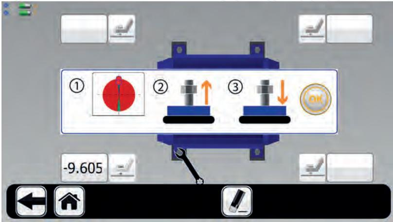
First loosen the chosen bolt completely, then tighten it firmly. It is recommended to use a torque wrench for tightening.
