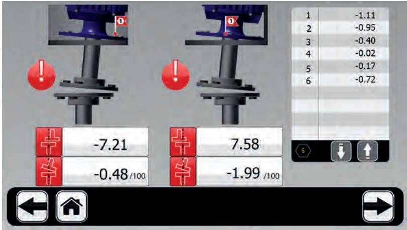
The table on the right contains bolts numbers with designation of shims required for eliminating misalignment.
