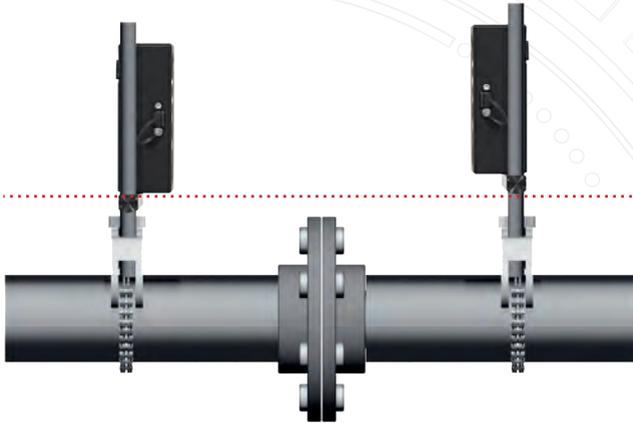
**The sensor units should be fixed with a shift (see the figure).**
