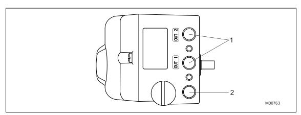
Fig. 23: Pneumatic connections
