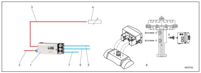
Fig. 21: TZIDC for remote position sensor
