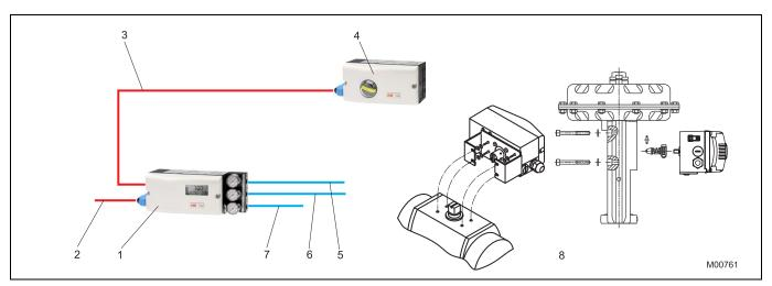
Fig. 19: TZIDC with remote position sensor
