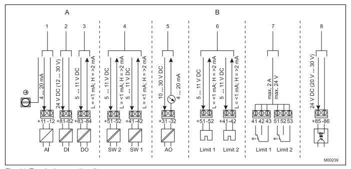
Fig. 14: Terminal connection diagram
