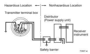
Figure 6.10 Connection between Transmitter and Distributor
