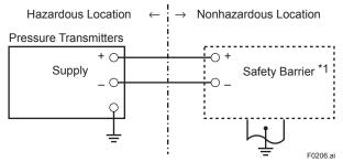
\*1: In any safety barriers used the output current must be limited by a resistor "R" such that Io=Uz/R.
