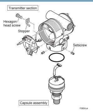
Figure 8.4 Removing and Mounting the Pressuredetector Section
