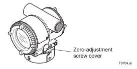
Figure 7.4 **External Zero-adjustment Screw**
