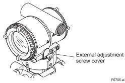
Figure 7.5 External Adjustment Screw
