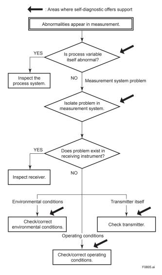
Figure 8.5 Basic Flow and Self-Diagnostics
