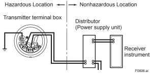
Figure 6.9 Connection between Transmitter and Distributor
