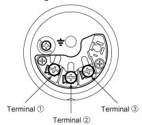
Terminal Wiring for 4 to 20 mA output,
