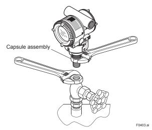
Figure 4.3 Tightening Transmitter
