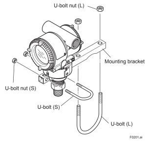
Figure 2.1 Transmitter Mounting Hardware
