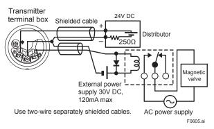
Figure 6.8 Status Output Connection
