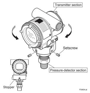
Figure 4.4 Rotating Transmitter Section
