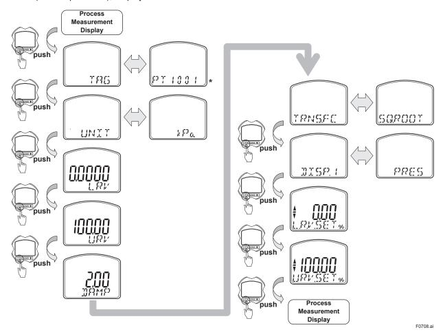
\*: Up to 6 characters are shown in the bottom line. To review after the 7th character, turn the external adjustment screw and press the push button six times or more.
