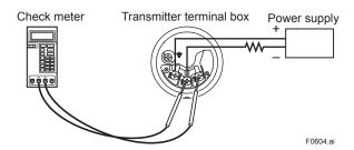
Figure 6.7 Check Meter Connection
