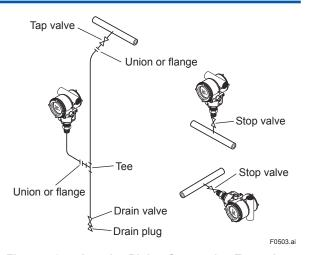
Figure 5.3 Impulse Piping Connection Examples
