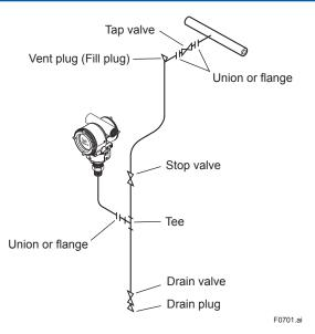
Figure 7.1 Liquid Flow Measurement (Gauge Pressure Transmitters)
