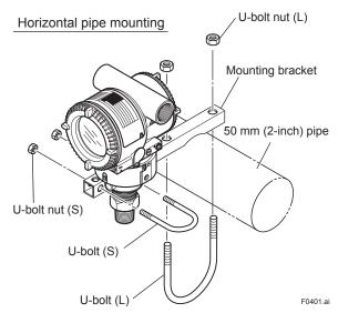
Figure 4.1 Transmitter Mounting
