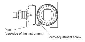
If the zero-adjustment screw is positioned other than donwards after installation, rotate the housing unit it is positioned downwards.
