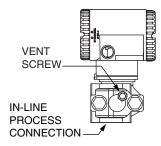
Figure 21. Horizontal Mounting - Cavity Venting and Draining
