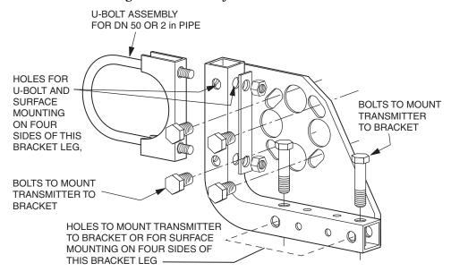
Figure 13. Details of a Universal Bracket
