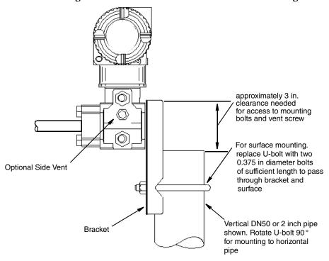
Figure 26. IAP20 and IGP20 Transmitter Mounting
