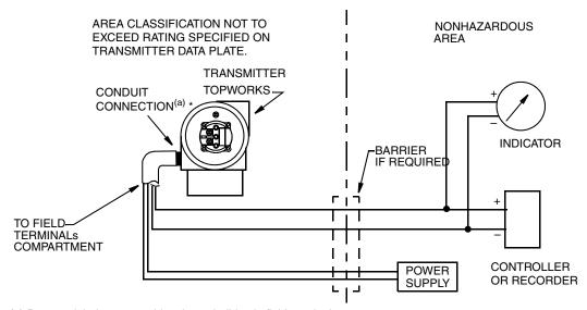
Figure 39. Loop Wiring (four-wire connection shown)
