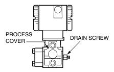
Figure 18. Vertical Mounting - Cavity Venting
