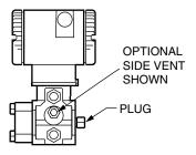
Figure 19. Horizontal Mounting - Cavity Venting
