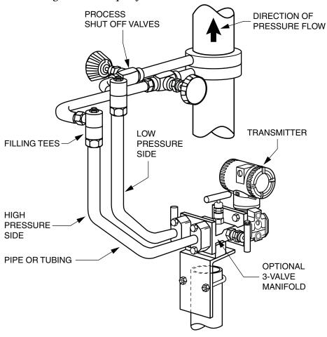
Figure 24. Example of Vertical Process Line Installation
