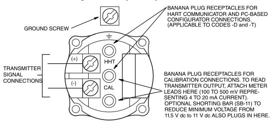
The transmitter is equipped with an internal ground connection within the field wiring compartment and an external ground connection at the base of the electronics housing. To minimize galvanic corrosion, place the wire lead or terminal between the captive washer and loose washer on the external ground screw.
