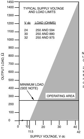
Figure 32. Supply Voltage and Loop Load
