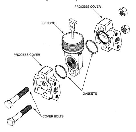
Figure 5. Sensor Replacement (pvdf Inserts)
