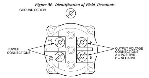
The transmitter is equipped with an internal ground connection within the field wiring compartment and an external ground connection at the base of the electronics housing. To minimize galvanic corrosion, place the wire lead or terminal between the captive washer and loose washer on the external ground screw.
