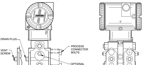
Figure 3. Pressure Connections
