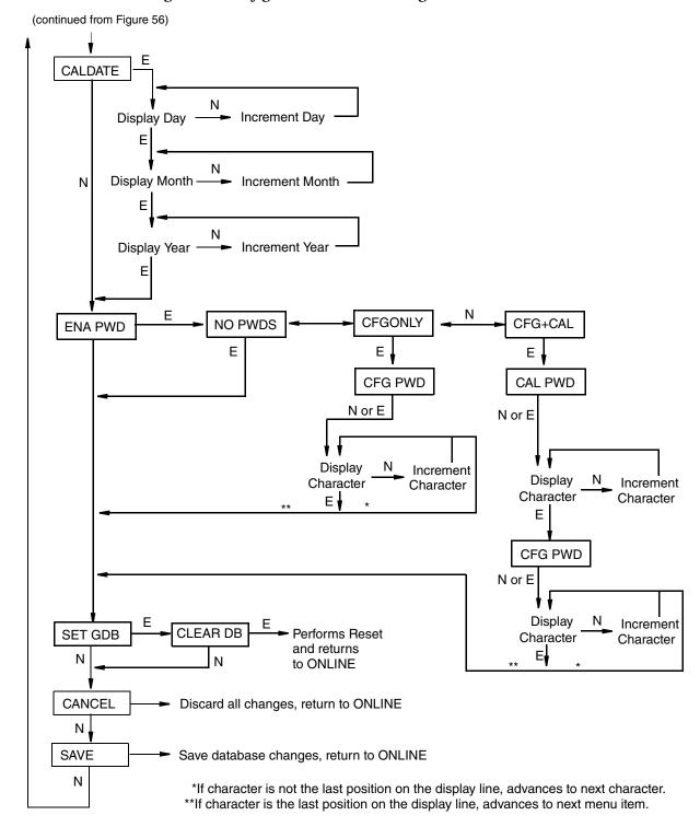
Figure 57. Configuration Structure Diagram (Continued)
