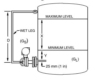
$\begin{aligned} & Span = (X)(G_L) \\ & LRV = Y(G_L) - D(G_S) \\ & URV = (X+Y)(G_L) - D(G_S) \\ & Range = LRV \text{ to } URV \end{aligned}$
