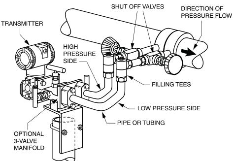
Figure 23. Example of Horizontal Process Line Installation
