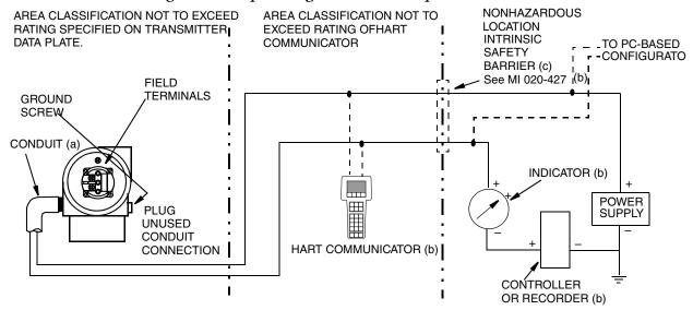
Figure 33. Loop Wiring 4 to 20 mA Output Transmitters
