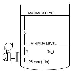
$\begin{aligned} & Span = (X)(G_L) \\ & LRV = (Y)(G_L) \\ & URV = (X+Y)(G_L) \\ & Range = LRV \text{ to } URV \end{aligned}$
