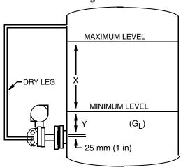
$Span = (X)(G_L)$   $LRV = (Y)(G_L)$   $URV = (X+Y)(G_L)$  Range = LRV to URV
