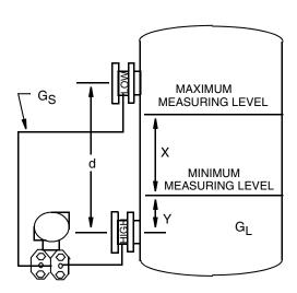
Figure 51. Transmitter Connected to Closed Tank With Dual Seals
