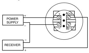
For wiring runs with high resistance due to long lengths or other reasons) or for maximum accuracy, a four-wire connection as shown in Figure 38 can be used to provide input-output isolation. With four-wire configuration, voltage drop in the power supply loop does not affect measurement accuracy.
