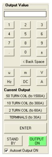
The output panel, shown left, allows the user to select a value to output and then automatically set the calibrator output and switch to the appropriate terminals / coil output on the workstation adapter.
