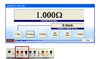
Connect meter to terminals marked continuity resistance.
