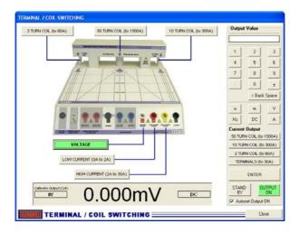
This function allows the calibrator output to be controlled for voltage and either direct current or current via the 2/10/50 turn coil. The current output can be routed through the coil for clamp meter calibration.
