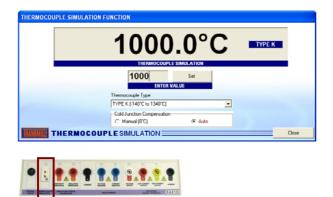
Connect temperature meter to thermocouple connector on workstation. Select a thermocouple type from the drop down list. Set manual or automatic cold junction.
