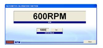
Enter an RPM value in the box marked ENTER VALUE, the press the SET button. The tachometer LED will illuminate – point the optical tachometer at the LED.
