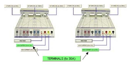
Note : Only the outputs which are available for current value entered are enabled – if the button is not available (greyed out) this means it is not possible to output this value using that specific output (eg. It is not possible to output 2A using the 50 turn coil – minimum value from 50 turn coil is 100A : 2A x 50 turns).
