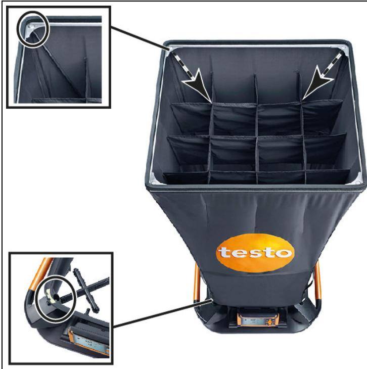
1. Lift the hood at the aluminum frame on
