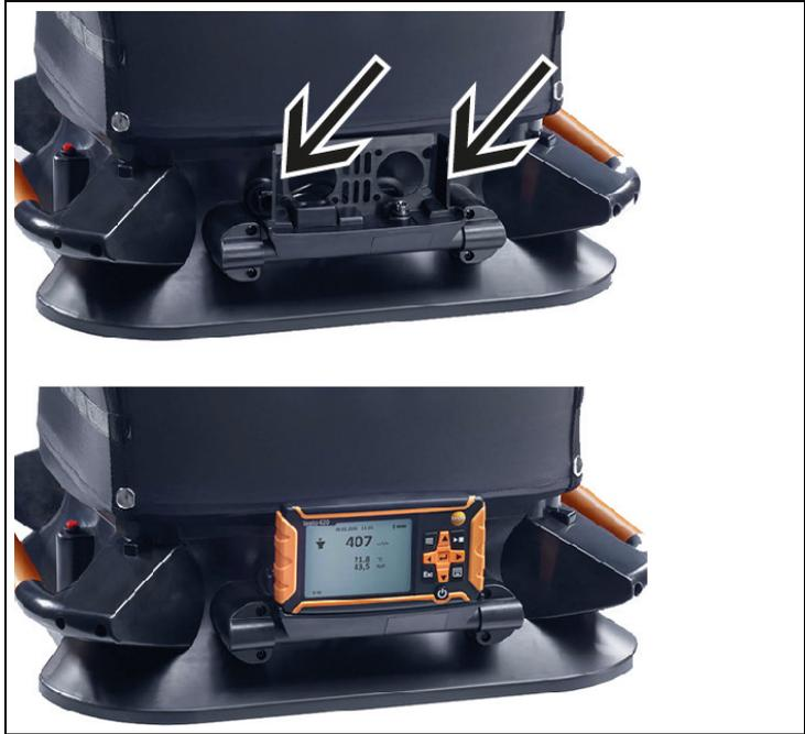
1. Make sure that the testo 420 is fully pushed into the instrument holder. In doing so, pay attention to the catch on the right-hand and left-hand side in the bracket.
