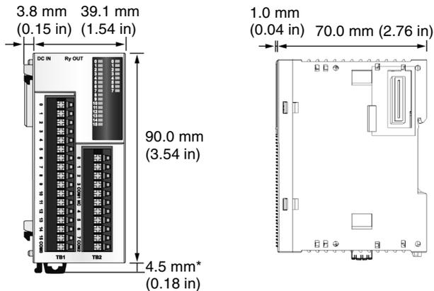
**Note:** \* 8.5 mm (0.33 in) when the clamp is pulled out.
