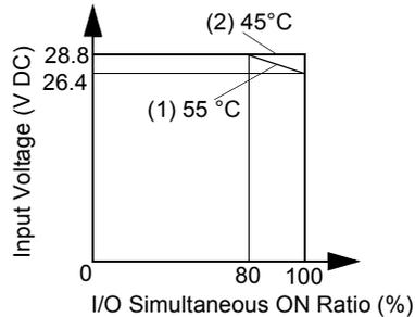
When using TWDDMM8DRT, all inputs and outputs can be turned on simultaneously at 55°C (131°F), input voltage 28.8 VDC.
