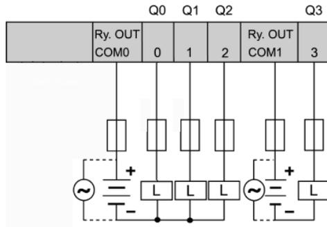
This schematic is for the TWDLC•A16DRF series controllers.
