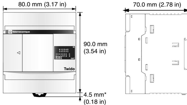
**Note:** \* 8.5 mm (0.33 in) when the clamp is pulled out.
