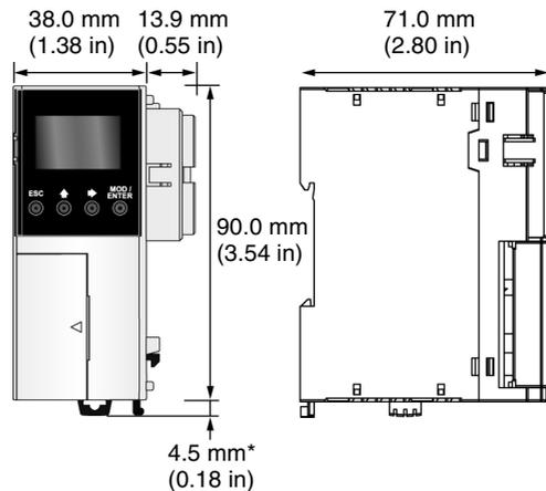
**Note:** \* 8.5 mm (0.33 in) when the clamp is pulled out.
