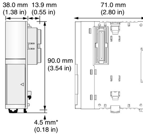
**Note:** \* 8.5 mm (0.33 in) when the clamp is pulled out.
