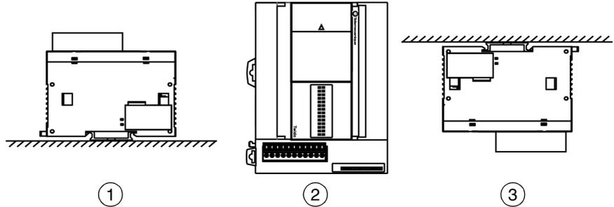
**Incorrect Mounting Positions for the Modular Controllers**
