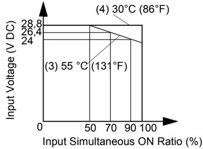
When using TWDDDI8DT, all inputs can be turned on simultaneously at 55°C (131°F), input voltage 28.8 VDC.
