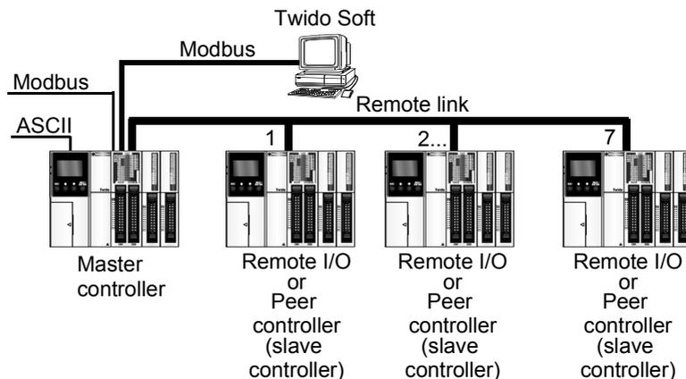
**Note:** Communication between the "Modbus" and "Remote Link" protocols cannot occur at the same time.
