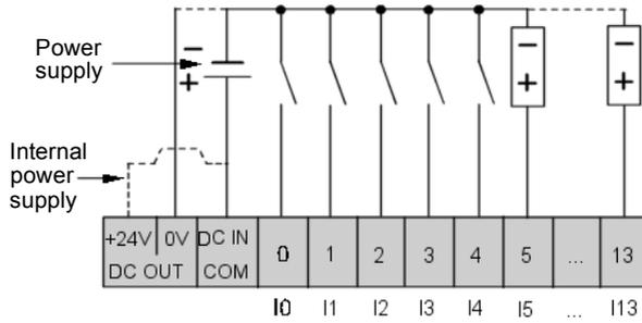
The following DC source input wiring schematic is for the TWDLCA•40DRF series controllers.
