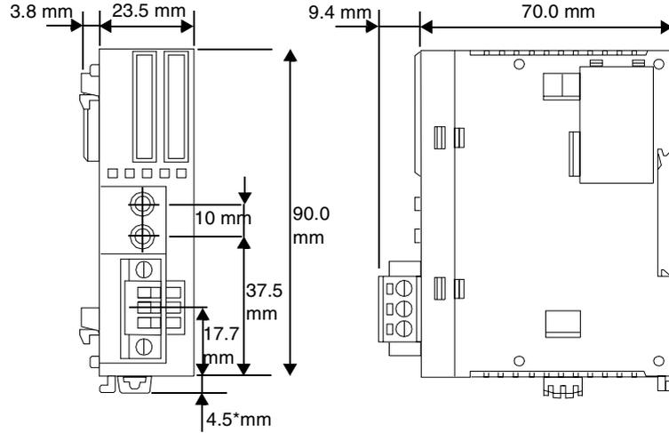
**Note:** \* 8.5 mm (0.33 in) when the clamp is pulled out.
