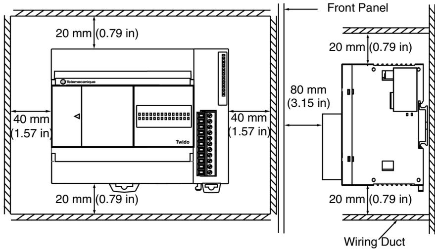
**Minimum Clearances for a Modular Controller and Expansion I/O Modules**
