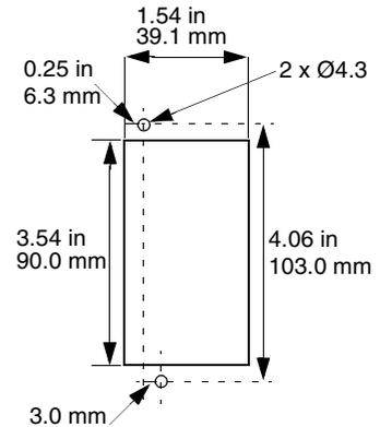
**Mounting Hole Layout for the AS-Interface Bus Interface Module**
