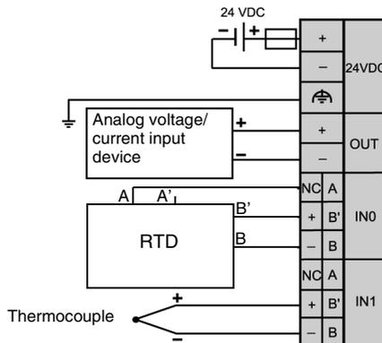
**Note:** For 4-wire cabling, output A' is not connected.
