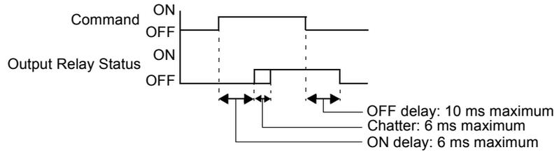
**Relay Output Contact** The relay output contact is shown below.
