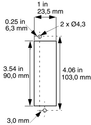
**Mounting Hole Layout for Communication Expansion and Operator Display Expansion Modules**
