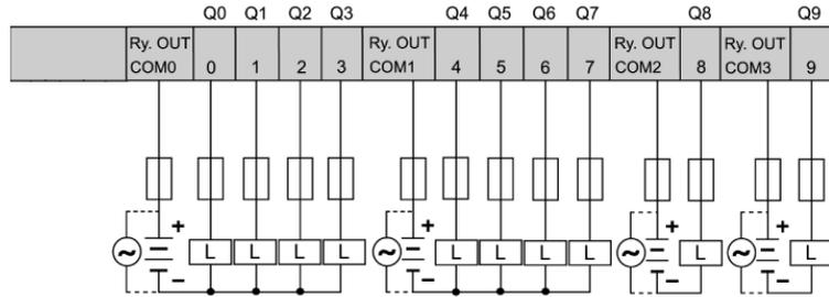
This schematic is for the TWDLCA•40DRF series controllers.
