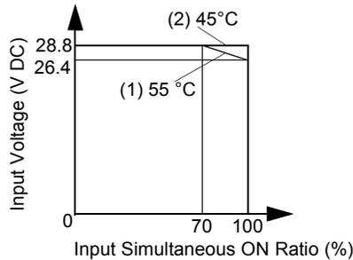
When using TWDDDI16DK and TWDDDI32DK at 55°C (131°F), limit the inputs which turn on simultaneously on each connector along line (3). This limitation applies per connector. At 30°C (86°F), all inputs can be turned on simultaneously at 28.8 VDC as indicated with line (4).
