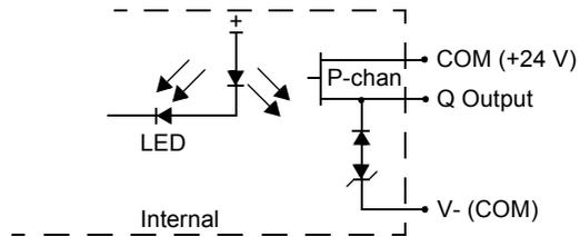
**Transistor Sink Output Contact**
