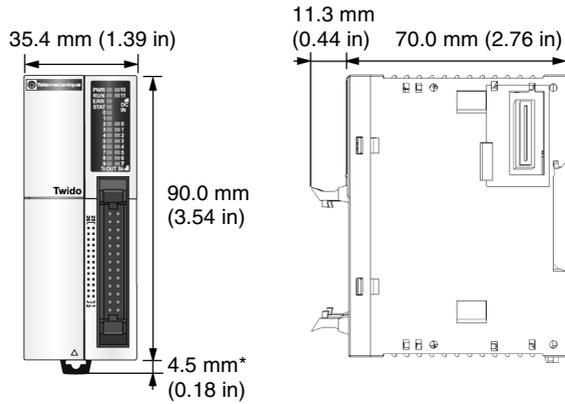
**Note:** \* 8.5 mm (0.33 in) when the clamp is pulled out.
