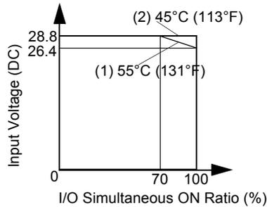
Also, when using the above-mentioned controllers at 45°C (113°F), all I/O can be turned on simultaneously at input voltage 28.8 VDC as indicated with line (2). When using the TWDDMM8DRT controller, all inputs and outputs can be turned on simultaneously at 55°C (131°F), input voltage 28.8 VDC. For other possible mounting directions, see *Controller, Expansion I/O Module and AS-Interface Bus Master Module Mounting Positions*, p. 178.
