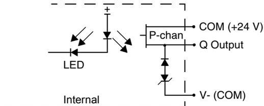
**Transistor Sink Output Contact**
