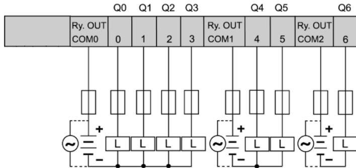
This schematic is for the TWDLC•A24DRF series controllers.
