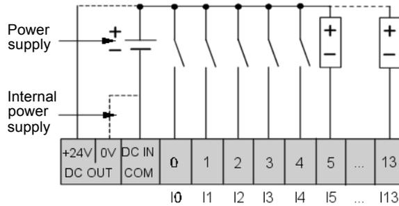
The following DC sink input wiring schematic is for the TWDLCA•40DRF series controllers.
