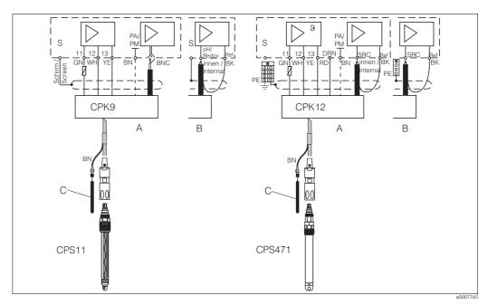
Connection CPS11 with CPK9 and CPS471 with CPK12 to Liquisys  ${\it M}$
