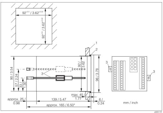
$In stall at ion\ of\ the\ panel-mounted\ in strument$
