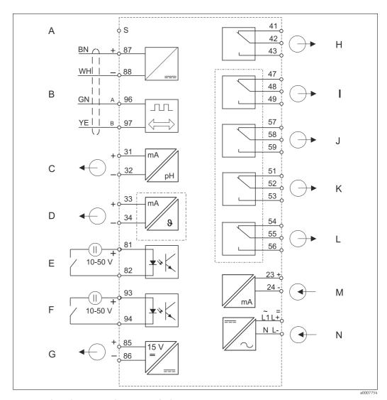
$Transmitter\ electrical\ connection\ with\ Memosens\ technology$
