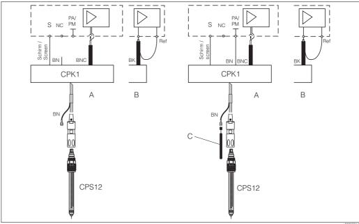
Unsymmetrical and symmetrical connection of ORP electrodes to Liquisys  ${\it M}$
