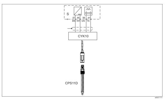
${\it Connection of digital sensor CPS11D with CYK10}$
