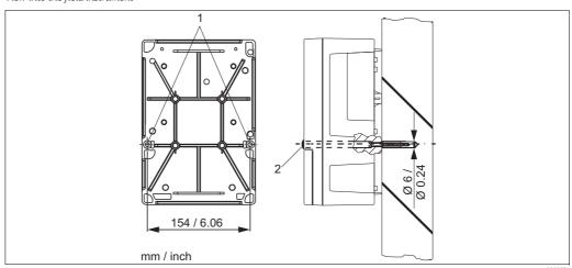
Wall mounting of the field instrument
