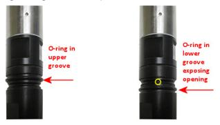
Be sure to move the o-ring to the lower groove before deploying, thus exposing the liquid junction port.
