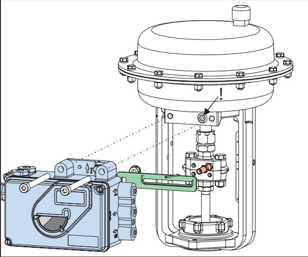
The attachment of the positioner is accomplished by bolting it directly to the actuator yoke using the feedback lever for a direct mount (with attachment kit EBZG -D).
