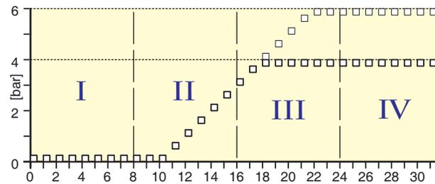
The pneumatic works precisely, if the actuator begins movement in section II and runs latest in section IV into the end position.
