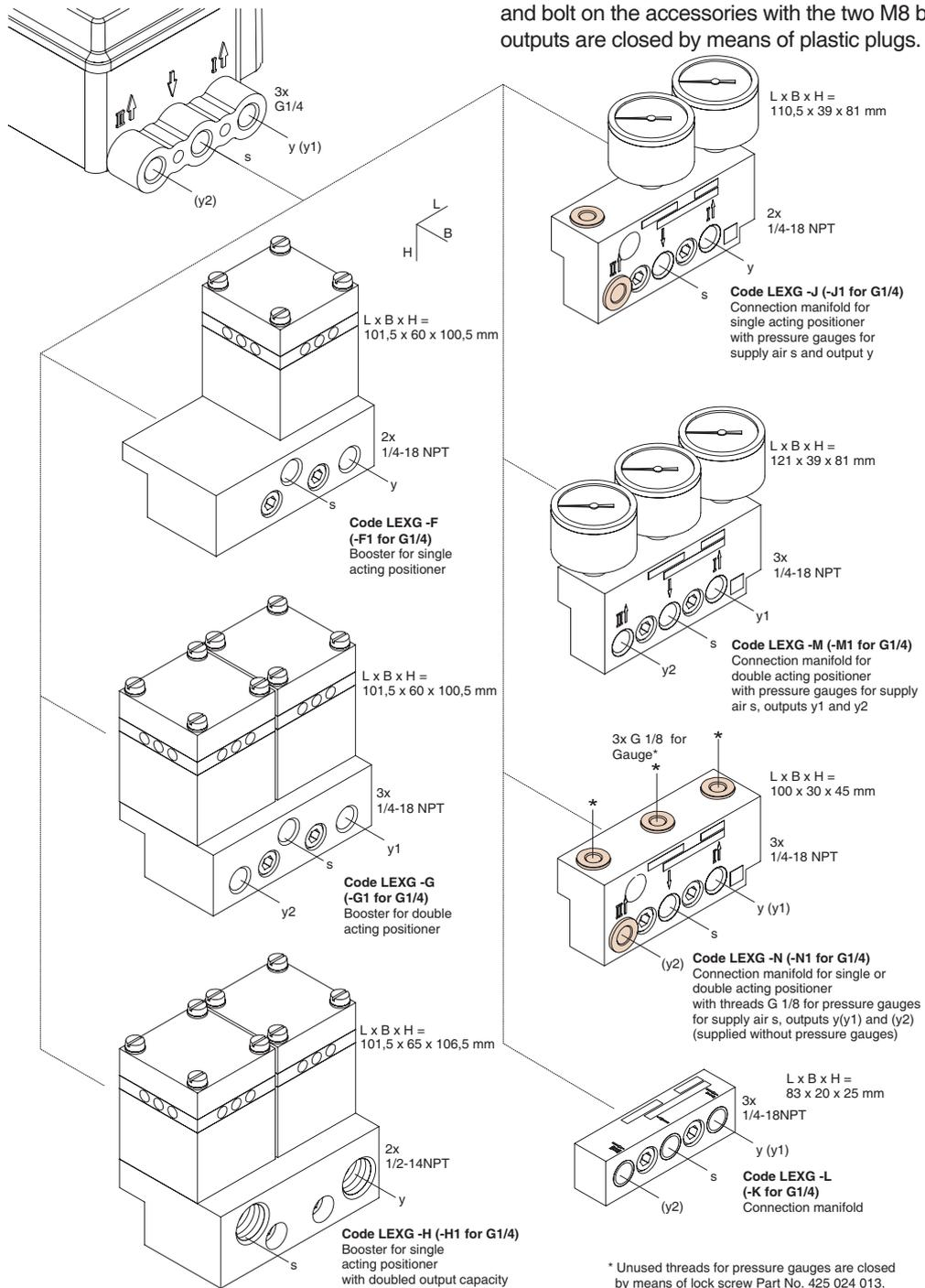
\* Unused threads for pressure gauges are closed by means of lock screw Part No. 425 024 013.
