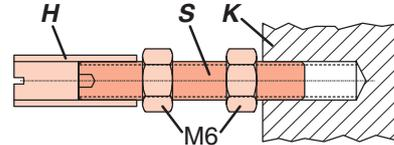
It consists of a stud S, which is screwed into the coupling piece K (with 3 mm Allen key) and locked with a lock nut M6. The threaded sleeve H is screwed onto it and locked with a lock nut M6. Make sure that the bolt is adjusted to the right length!
