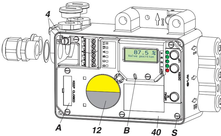
If the SRD is equipped with option “IrCom” **B**, communication can take place contactless via infrared with the positioner (even with closed cover!). Modem “IR Interface” (not Ex) is connected via RS232 to a PC (for practical reasons a notebook) with software PC20 / PC50 and makes possible a range of approx. 1 m.
