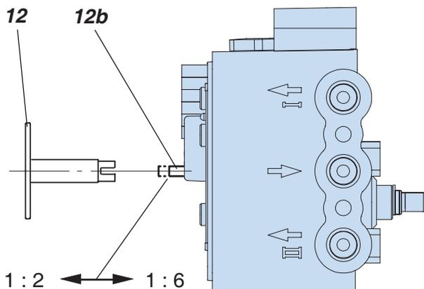
Turn the travel indicator **12** to the desired position, put it on the gear shaft against the stop and pinch the wire ring for secure coupling.
