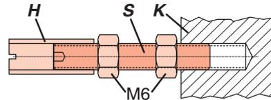
It consists of a stud **S**, which is screwed into the coupling piece **K** (with 3 mm Allen key) and locked with a lock nut M6. The threaded sleeve **H** is screwed onto it and locked with a lock nut M6. Make shure that the bolt is adjusted to the right length!
