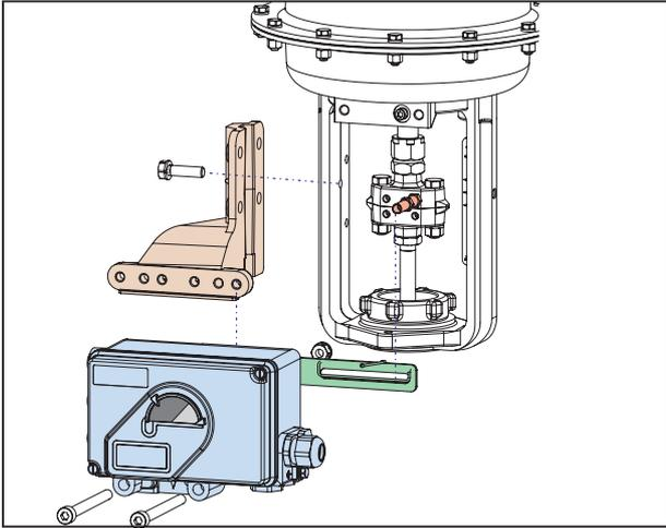
Attachment of the positioner to the actuator is made to the left using the mounting bracket and feedback lever for a NAMUR mount. Use:
