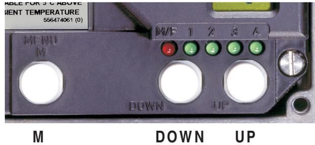
If there is no response using the local key-pad (message 1 appears, see page 50) make sure that the Write Protection is not set ! Remove the write protection using the configuration software (PC20 / IFDC or PC50 (FDT) software).
