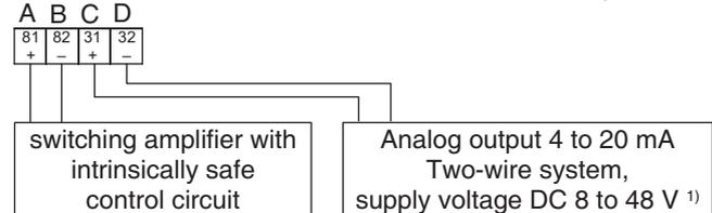
1) For intrinsically safe circuits please refer to certificate / data plate for max. operating voltages etc.
