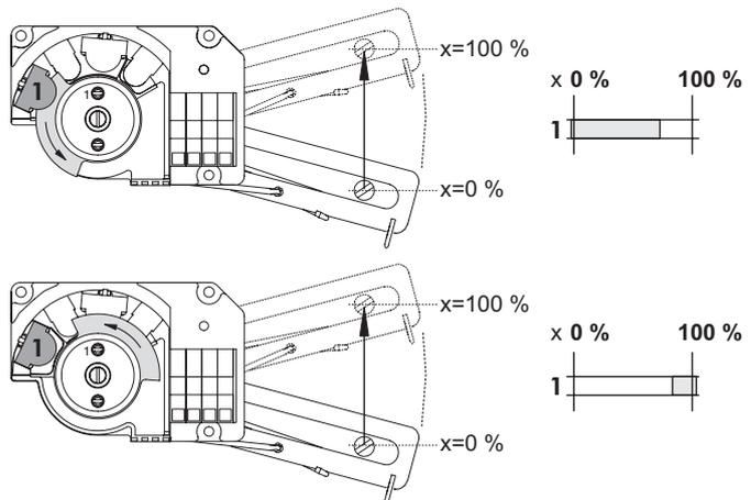
**Setting limit switch trigger points**
