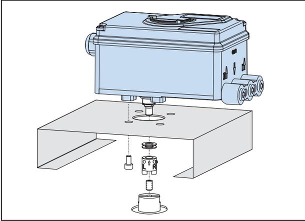
**Attention:** The feedback shaft **9** of the SRD has no mechanical stop, therefore may spin 360 degrees. The permissible rotation angle range is between +50 and -50 degrees around the arrow at the housing concerning the flat area of the feedback shaft (also see detail page 17 bottom). Since a rotary actuator has a rotary angle of about 90 degrees the mounting as described in the following must be carried out very precisely.
