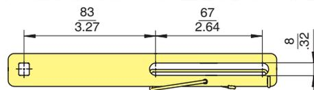
**Carrier bolt** for connection to valve stem
