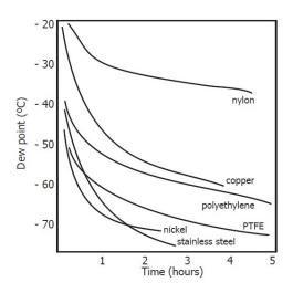
Figure 11 Material Permeability Comparison
