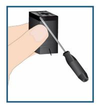
Figure 1 Connector Terminal Block Removal
