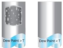
If temperatures drop below the sample dew point, water may condense in sample tubing and affect the accuracy of measurements.
