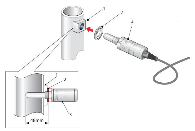
Figure 12 Transmitter Mounting - Pipe or Duct
