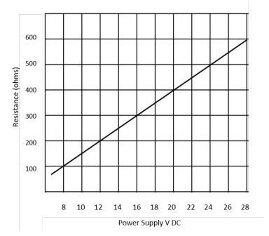
Figure 7 Maximum Load of SF82 - Including Cable Resistance
