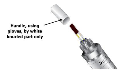
Figure 14 Replacement HMWPE Guard
