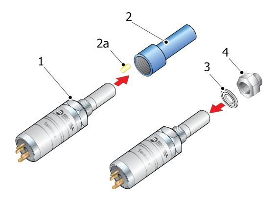
Figure 13 Transmitter Mounting with Adapter
