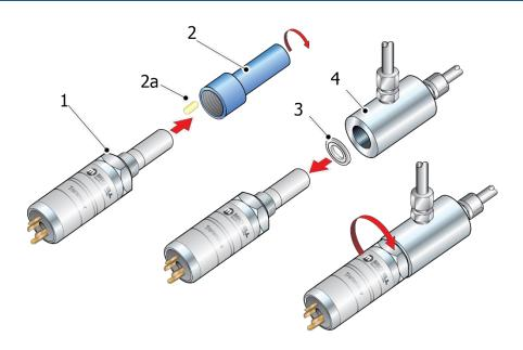
Figure 10 Transmitter Mounting - Sensor Block
