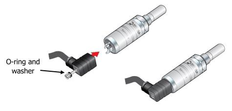
Figure 5 Connector Installation
