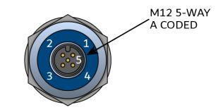
Figure 3 Sensor Connector Installation
