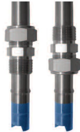
Figure 44. The 23166-00 (or -01) metal process connector, shown with the 3300HT PERpH-X sensor, allows various insertion depths, depending on where the user locates the compression fitting. Also the threads can be switched to face the top end of the sensor (right) for connection to submersion pipes.
