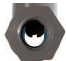
Figure 13. Sensor tip in process stream flow path.
