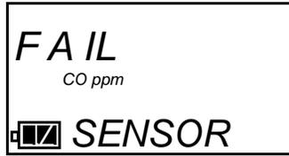
If you wish to continue, press and release the POWER MODE button to acknowledge the failure. The gas reading for the failed sensor will be replaced by “- - -”. Replace the failed sensor as soon as possible.
