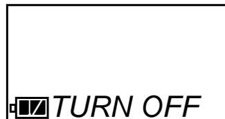
5. Press and hold the POWER MODE button until the unit turns off, then release it. Recharge the GX-2009's batteries. See "Recharging the GX-2009's NiMH Batteries" on page 52.
