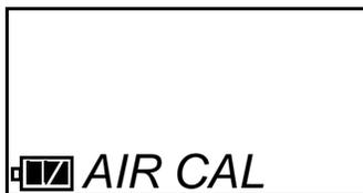
Perform a fresh air adjustment in Calibration Mode when you are performing a calibration before proceeding either to the AUTO CAL or ONE CAL menu item to perform a span adjustment. A fresh air adjustment performed in Calibration Mode is the same as a fresh air adjustment in Normal Mode. The AIR CAL menu item is available in Calibration Mode for convenience when performing a complete calibration.
