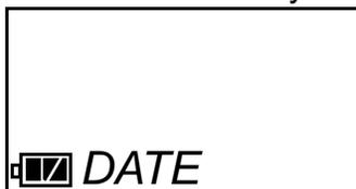
1. When the DATE Screen is displayed, press and release the POWER MODE button. A screen appears with the year flashing in the upper left, the month and day in the upper right, and the time in the lower right.
