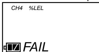
In this example, the CH<sub>4</sub> channel failed the span adjustment. Press and release the POWER MODE button to clear the failure indication and return to the AUTO CAL screen.
