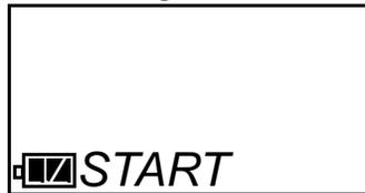
7. At the START screen, press and release the POWER MODE button. The GX-2009 will begin its start-up sequence.
