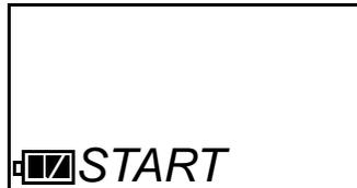
10. At the START screen, press and release the POWER MODE button. The GX-2009 will begin its start-up sequence.
