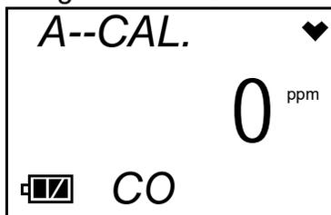
If you want to cancel the calibration, press and hold the AIR key for 2 seconds. The instrument will return to the A--CAL. Screen. If you hold the AIR key down longer than 2 seconds, the instrument will start scrolling through the Calibration Mode items.
