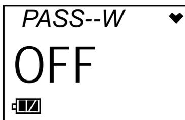
2. Press and release the AIR button to change the displayed setting. When the desired setting is displayed, press and release the POWER MODE button to save the setting.
