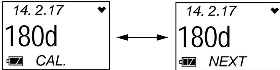
**NOTE:** The following screens in Step 6 only appear if **Bump Test Limit Display** is set to *On* using the 03 Series User Setup Program. The standard factory setting for this function is *Off*.
