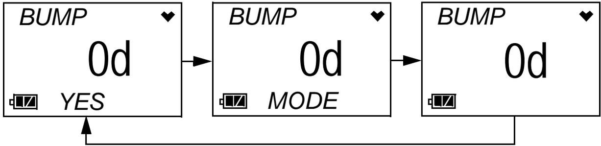
Press and release the POWER MODE button during this time to go to the BUMP menu item in Calibration Mode. If no button is pressed, the instrument will continue with the warmup sequence in Step 8 once the sequence shown above has finished.
