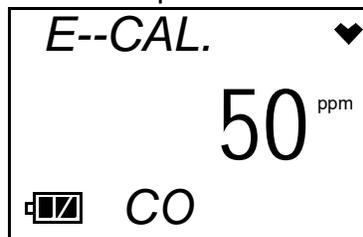
3. Press and release the POWER MODE button. The LCD will display the current gas readings and “E--CAL.” will flash.
