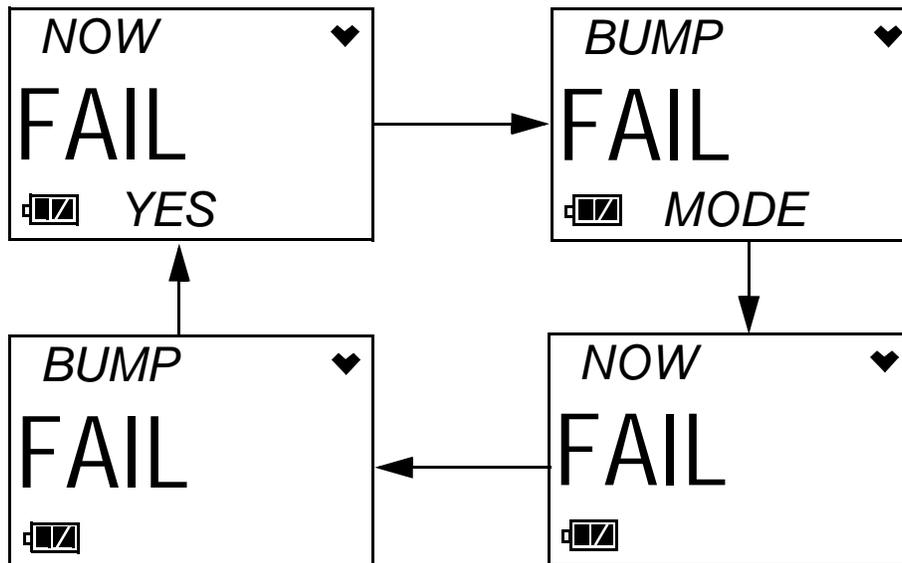
The alarm LED and buzzer will pulse several times. Press and release the POWER MODE button to go to the BUMP menu item in Calibration Mode. The above screens will remain on the display until the unit is either turned off or Calibration Mode is entered. The 03 Series cannot be used until a bump test has been performed. See “Performing a Bump Test in BUMP” on page 53 for bump test instructions.
