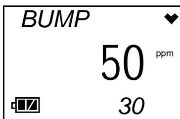
If the value is not correct, you can change it by changing the A--CAL gas value in Calibration Mode or Setup Mode or by using the 03 Series Data Logger Management Program or the 03 Series User Setup Program.
