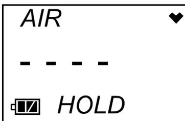
4. Release the AIR button when the following screen appears.
