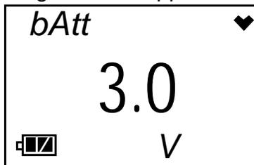
The screen displays the current battery voltage.
