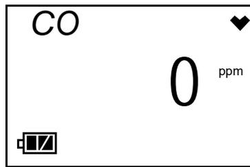
The gas concentration of the target gas is displayed along with the battery charge level in the lower left corner. The heart symbol displayed in the upper right corner flashes while the instrument is functioning properly. If it disappears or is steadily on, the unit is experiencing a microprocessor error. The backlight turns off after 20 seconds.
