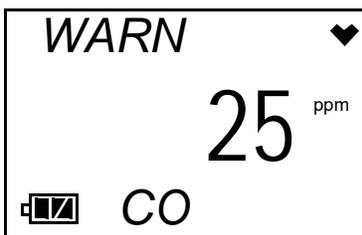
2. Use the AIR button to adjust the Warning setpoint to the desired value.
