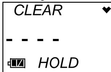
Hold the AIR button until the following screen appears, then release it.
