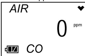
If you want to cancel the fresh air adjustment, press and release the AIR button to return to the AIR screen. To continue with the fresh air adjustment, proceed to Step 3.
