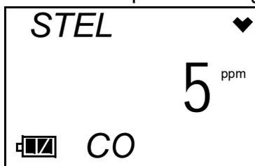
7. Use the AIR button to adjust the STEL setpoint to the desired value.
