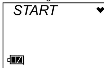
7. At the START screen, press and release the POWER MODE button. The 03 Series will begin its start-up sequence.
