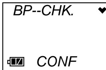
2. Use the AIR button to scroll through the options. CONF is the factory setting.
