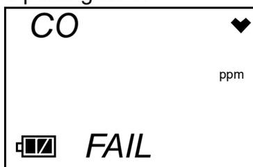
Press and release the POWER MODE button to clear the failure indication and return to the E--CAL. screen.
