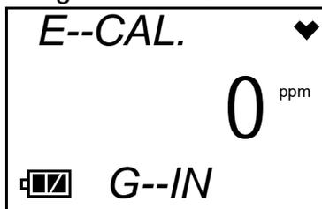
If you want to cancel the calibration, press and hold the AIR key for 2 seconds. The instrument will return to the E--CAL. Screen. If you hold the AIR key down longer than 2 seconds, the instrument will start scrolling through the Calibration Mode items.
