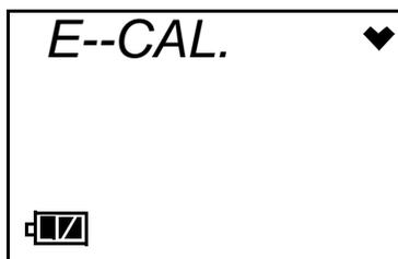
Perform a span adjustment (zero adjustment for OX-03) as part of a calibration after performing a fresh air adjustment. Performing a span adjustment (zero adjustment for OX-03) requires the use of a calibration kit. A calibration kit is available from RKI Instruments, Inc. for each 03 Series model (see “Parts List” on page 76). You will need:
