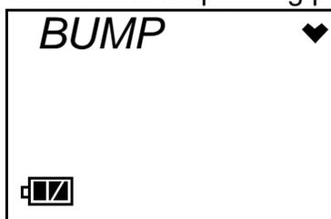
Performing a bump test requires the use of a calibration kit. A calibration kit is available from RKI Instruments, Inc. for each 03 Series model (see "Parts List"). You will need:
