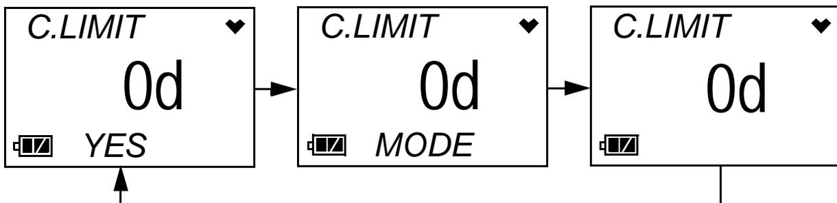
Press and release the POWER MODE button during this time to go to the A--CAL or E--CAL menu item in Calibration Mode depending on the value entered into the **One Touch Cal Time** parameter of the 03 Series User Setup Program. If no button is pressed, the instrument will continue with the warmup sequence in Step 6 once the sequence shown above has finished.
