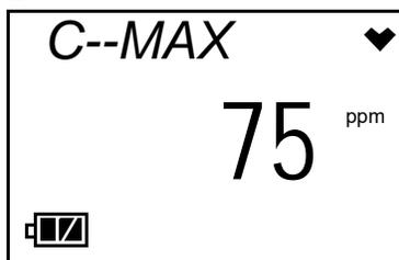
11. If the span adjustment (zero adjustment for OX-03) fails, the LCD will show the following screen, the alarm LED will flash, and the buzzer will sound a double pulsing tone.
