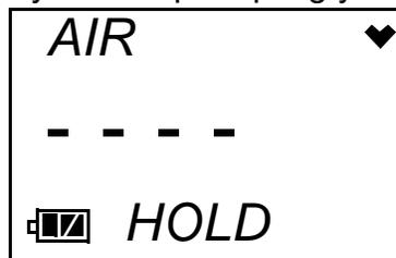
3. Release the AIR button when the following screen appears. The unit will set the reading to 0 ppm (20.9% for the OX-03) and return to Measuring Mode.
