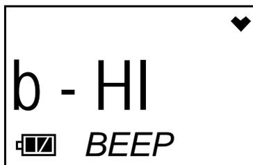
3. Use the AIR button to select LO or HI. The buzzer volume during the simulated alarm condition will change as you select a different volume.
