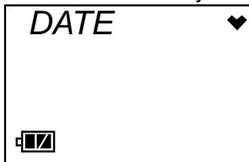
1. When the DATE Screen is displayed, press and release the POWER MODE button. A screen appears with the year flashing in the upper left, the month and day in the middle, and the time in the lower right.
