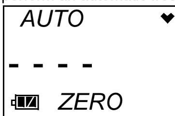
If the fresh air adjustment is successful, the unit will proceed to Normal Mode. If the sensor fails the air adjustment, the screen will indicate the failure. If a failure occurs, press and release the POWER MODE button to proceed to Normal Mode. Replace the failed sensor as soon as possible.
