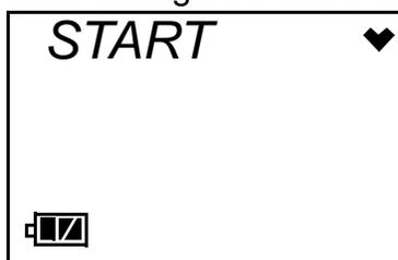
10. At the START screen, press and release the POWER MODE button. The 03 Series will begin its start-up sequence.
