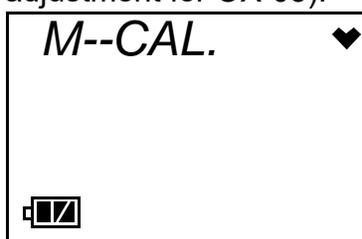
Perform a span adjustment (zero adjustment for OX-03) as part of a calibration after performing a fresh air adjustment. Performing a span adjustment (zero adjustment for OX-03) requires the use of a calibration kit. A calibration kit is available from RKI Instruments, Inc. for each O3 Series model (see “Parts List” on page 76). The procedure below describes a span adjustment (zero adjustment for OX-03). You will need:
