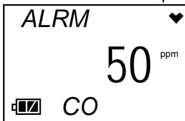
4. Use the AIR button to adjust the Alarm setpoint to the desired value.
