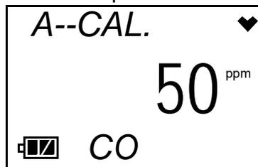
3. Press and release the POWER MODE button. The LCD will display the current gas readings and "A--CAL." will flash.
