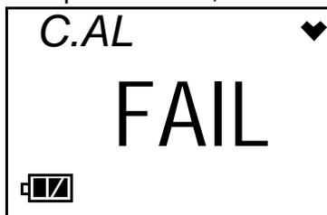
The instrument cannot be used until a successful bump test or calibration is performed. See “Calibration Mode” on page 36 for instructions.
