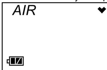
Perform a fresh air adjustment in Calibration Mode when you are performing a calibration before proceeding either to the A--CAL or M--CAL menu item to perform a span adjustment (zero adjustment for OX-03). A fresh air adjustment performed in Calibration Mode is the same as a fresh air adjustment in Normal Mode. The AIR menu item is available in Calibration Mode for convenience when performing a complete calibration.
