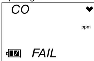
Press and release the POWER MODE button to clear the failure indication and return to the A--CAL. screen.
