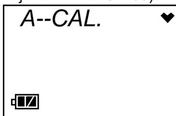
Perform a span adjustment (zero adjustment for OX-03) as part of a calibration after performing a fresh air adjustment. Performing a span adjustment (zero adjustment for OX-03) requires the use of a calibration kit. A calibration kit is available from RKI Instruments, Inc. for each 03 Series model (see “Parts List” on page 76). You will need:
