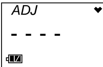
5. The unit will take a few seconds to adjust the fresh air reading, then indicate "END" in the upper left corner and return to the AIR Screen.
