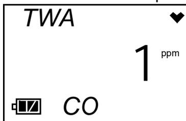
9. Use the AIR button to adjust the TWA setpoint to the desired value.
