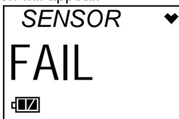
The instrument cannot be used if a sensor failure occurs. Replace the failed sensor.
