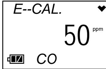
If the displayed concentration matches the calibration cylinder concentration, continue with Step 3.
