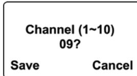
Step from digit to digit from left to right by pressing [MODE]. Change a digit's value by pressing [Y/+] to increase and [N/-] to decrease. When you press [MODE] you see a flashing "?" after the second digit:
