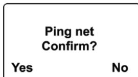
Press [Y/+]. The Echoview Host broadcasts a ping signal to its network. All devices in the network that receive the ping signal respond with a beep if they are within the range. (The Echoview Host does not beep or flash its LED lights.) You can also ping from an instrument in the network. If it is within range, the EchoView Host responds with a beep and an LED light flash.
