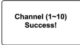
**Important!** Remember that the range of allowed channels for instruments on a EchoView Host's network depends on the wireless modem frequency. Therefore, you may not be able to change the channel to a number outside of its assigned set of numbers. If you select an incompatible channel number, you will see this screen, and then the EchoView Host returns to the Wireless menu.
