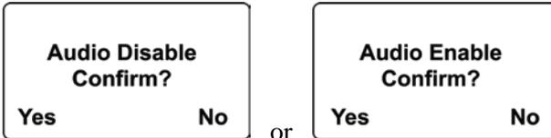
To toggle the audible alarm from on to off (or off to on), press [Y/+], and a confirmation message appears. To exit without performing the reset, press [N/-].
