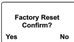
To perform the reset, press [Y/+]. To exit without performing the reset, press [N/-].
