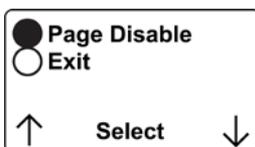
When the Page feature is enabled, the EchoView Host broadcasts instrument data. These data can be picked up by mimic panels. If no mimic panels are planned to be used, this feature should be disabled, in order to ensure data privacy. **Note:** The default value is “Disabled.”
