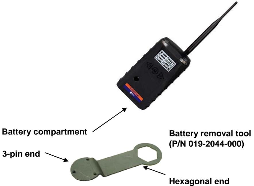
1. Use the 3-pin end of the tool to unscrew and open the battery cover by turning it counterclockwise.
