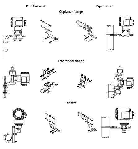
Figure 6. Common Transmitter Assemblies
