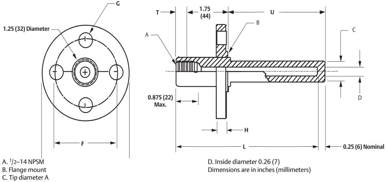
**Figure 39. Flange Mounted Thermowells - Tapered<sup>(1)</sup>**
