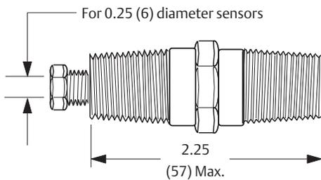
**Option Codes C01, C02, Swagelok® compression fitting**
