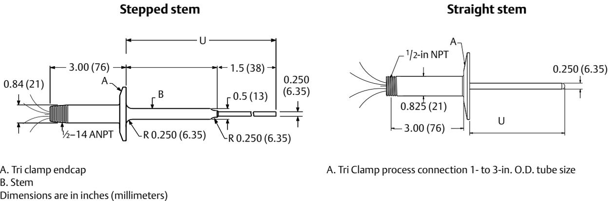
Figure 19. Rosemount 68Q Mini General Purpose Sensor with Cable and Strain Relief
