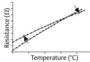
A two-point trim shifts the ideal curve up or down, and changes the slope based on the two characterized points.
