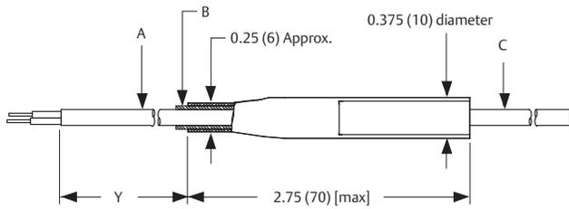
A. Shielded cable PTFE jacket 22-Gauge PTFE-Insulated wires
