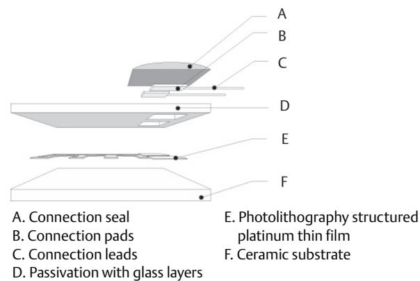
Design and construction of the Rosemount Series 68 Platinum Sensors provides the optimum combination of accuracy and durability available for temperature measurements. The construction of the sensor allows for direct immersion in non-corrosive fluids at reasonable static pressures. For corrosive environments or many industrial applications, these sensors are widely used with standard thermowell assemblies.
