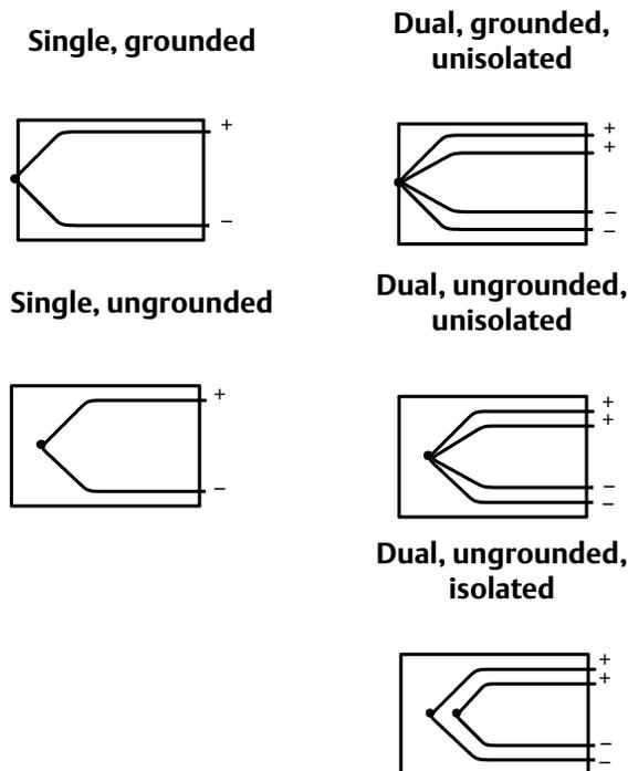
**Figure 16. Rosemount Series 183 Lead Wire Configurations**
