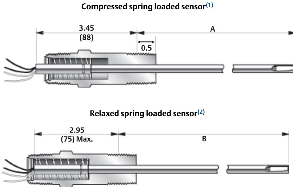
A. Installed (X) Length [Spring Compressed 0.5 (13) nominal]
