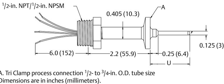
**Figure 21. Rosemount 68Q Mini Spring Loaded Sensor with Thermowell and Replaceable Sensor**
