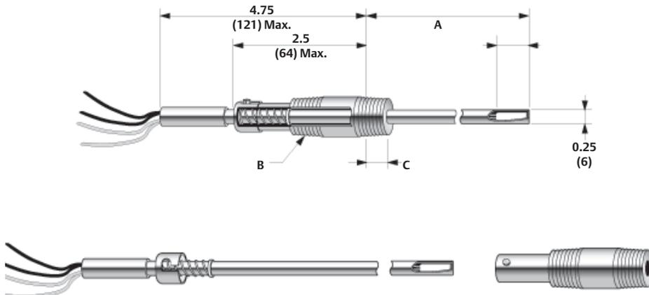
A. Installed (X) length [spring is shown compressed 0.5 (13)]
