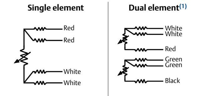
1. Dual element sensors are only available on Rosemount Series 68Q and 78 Sensors.
