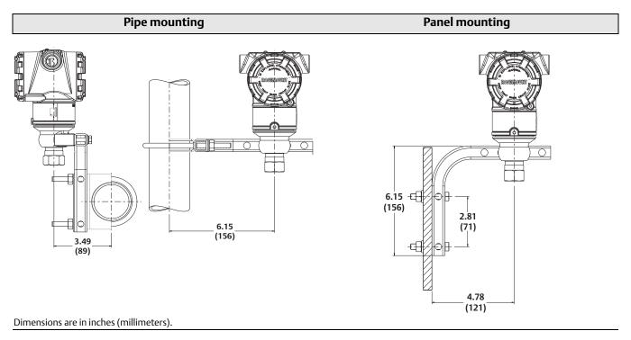
Figure 13. Rosemount 3051CFA Pak-Lok Annubar Flowmeter<sup>(1)</sup>
