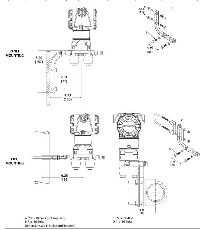
Figure 6. Rosemount 3051C Coplanar with Traditional Flange
