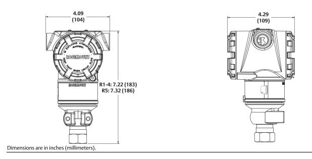
Figure 10. 3051T Wireless Housing Dimensional Drawings
