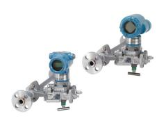
Rosemount 3051CFP Integral Orifice Flowmeters enable highly accurate flow measurement in small line sizes. Integral Orifice utilize precision honed pipe section for increased accuracy and self-centering plate design to prevent alignment errors that magnify measurement inaccuracies in small line sizes.
