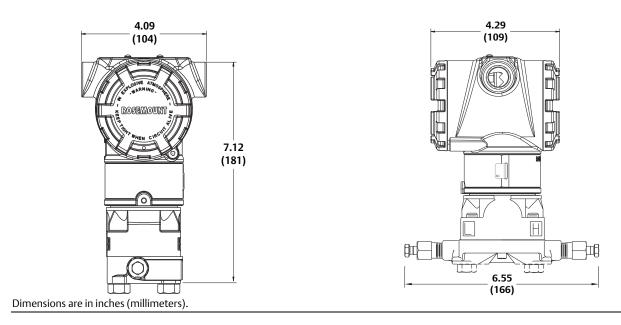
Figure 3. 3051 Wireless Housing with Coplanar Flange
