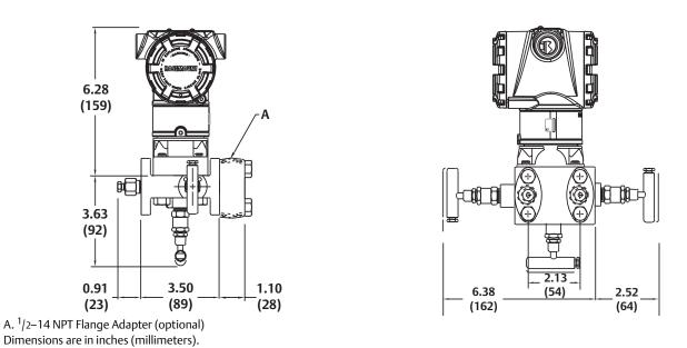
Figure 8. Traditional Flange Mounting Configurations with Optional Brackets for 2-in. Pipe or Panel Mounting
