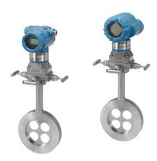
Rosemount 3051CFC Compact Flowmeters provide a quick, reliable installation between existing raised face flanges. Depending on your application needs, you can reduce energy loss with the Compact Annubar or minimize straight run requirements with the Conditioning Orifice.
