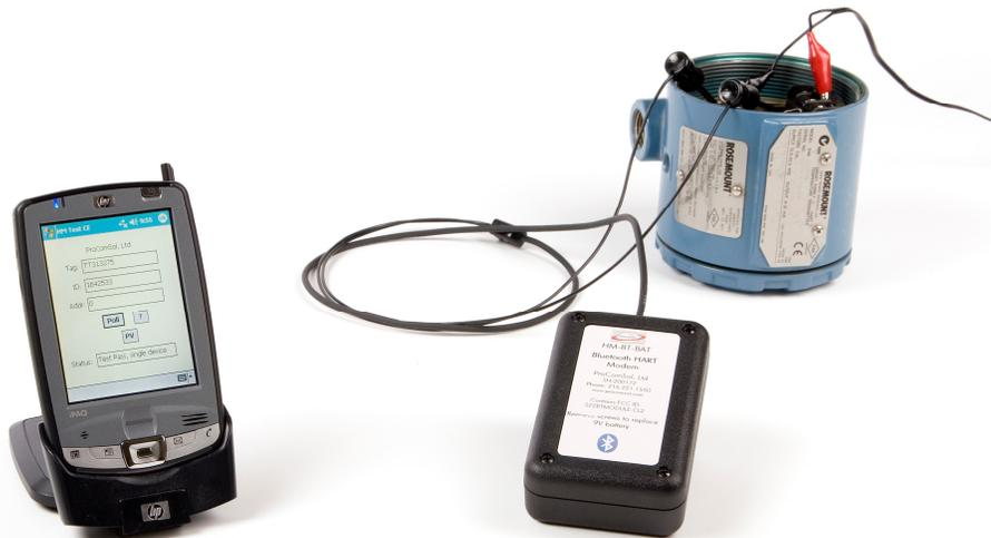
**Figure 1 Typical DevCom2000 Mobile Hardware Setup**
