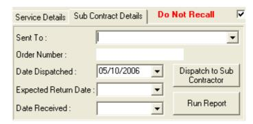
Select the sub-contractor from the "Sent To" list. Enter an order number and the expected return date, and then click "Despatch to sub contractor". The instrument status will be set to K – Sent for cal (External).
