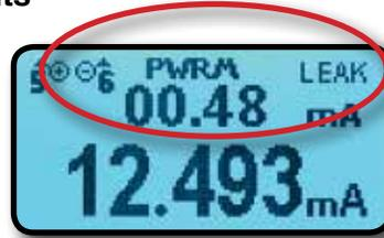
820-ELITE detects uncontrolled current in the loop due to a flooded junction box.
