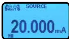
Source & Read 0.000 to 24.000 mA, Simulate a 2 Wire Transmitter or use the 820-ELITE to simultaneously power your 2 Wire Transmitter and measure its output.
