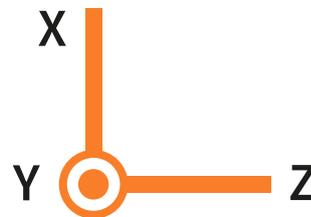
Once that you've placed the sensor on your machine, set it up on Digivibe and define each axis to an orientation: Horizontal, Vertical and Axial.
