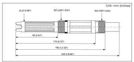
Figure 4. Dimensions of the sensor
