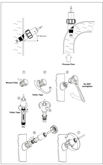
Figure 7. Sensor & adapter Installation
