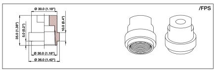
Figure 11. Dimensions FU20 adapter for FF40, FS40 and FD40 fittings
