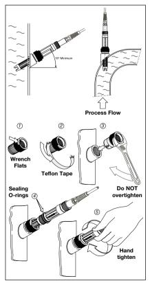
Figure 1. Sensor Installation
