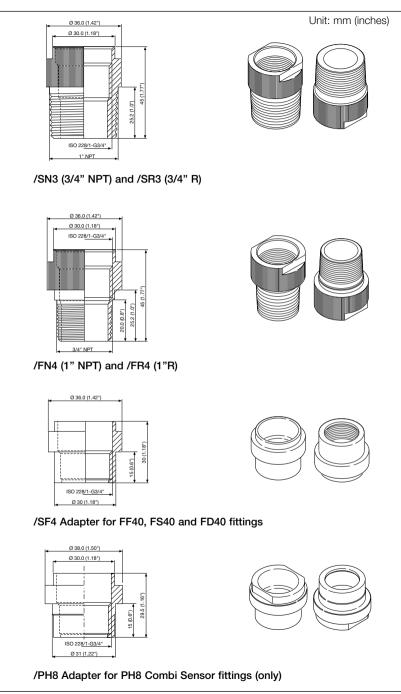
Figure 5. Dimensions of the adapters
