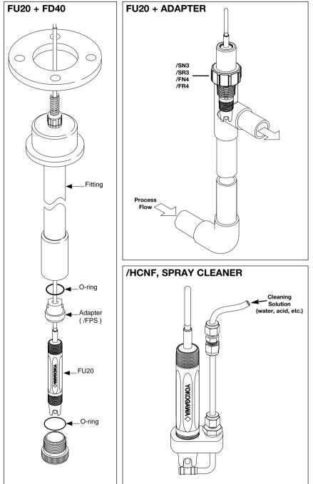
Figure 8. Installation examples for the FU20
