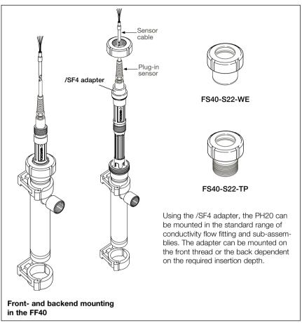
Figure 3. Installation Examples using the /SF4 adapter
