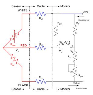
Figure 2-4: Monitor and Sensor Front End
