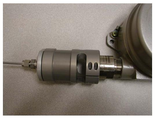
Figure 2-6 Remote Calibrator mounted on Haz Gas Sensor
