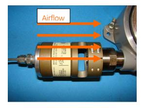
Figure 5-4: Sensor must face into high airflow (orientation of air intake opening of Remote Calibrator is not critical)
