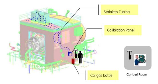
Figure 5-1 Example of remote calibrator installation
