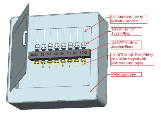
Figure 5-3: Example Interface Panel for Remote Calibrators
