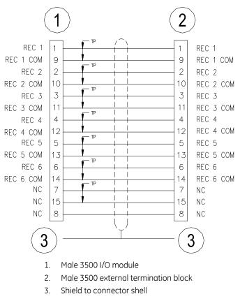
Figure 8-9: Recorder Terminal Block Wiring Diagram
