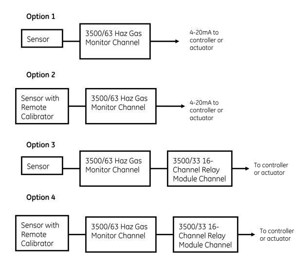
Figure 12-1: SIL Capable Configurations
