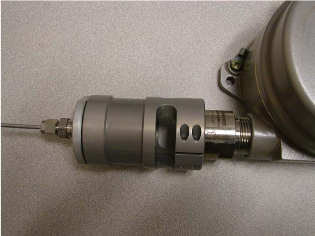
Figure 2-6 Remote Calibrator mounted on Haz Gas Sensor
