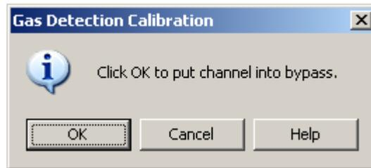
**Figure 9-9: Initiate Bypass for Calibration**
