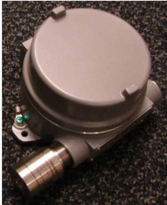
Figure 2-5: Sensor with Flameproof Housing
