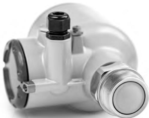
The small beam angle and negligible dead zone of this 80 GHz FMCW radar level transmitter makes it the premium choice for liquids in small and narrow tanks with internal obstructions like agitators or heating coils, as well as tanks with long nozzles. It can even measure through tank roofs made of non-conductive material (e.g. plastic, fiberglass or glass). The flush-mounted PEEK Lens antenna (no tank intrusion) is insensitive to deposit.
