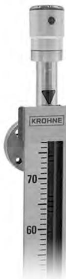
The OPTIWAVE 1010 is a non-contact FMCW radar welded to a bypass chamber with an optional IP68 level indicator (BM 26 Advanced). It continuously measures the distance and level of clean liquids.
