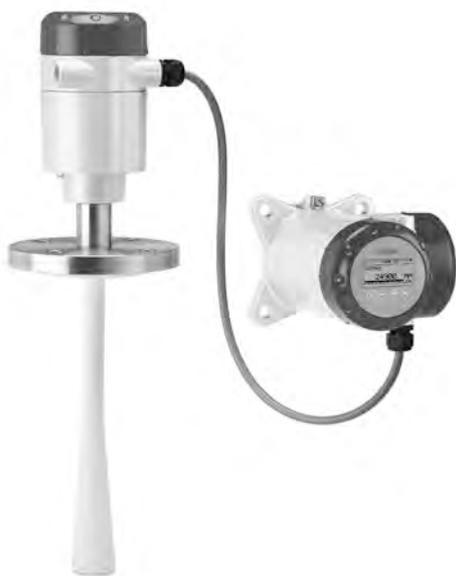
This 10 GHz 2-wire FMCW radar level transmitter measures distance, level, volume, mass and flow rate of liquids and pastes. It is ideal for corrosive products with its PP or PTFE antenna options. It features unique PP and PTFE antennas for aggressive products. The device is able to measure distances up to 30 m / 98.4 ft in process conditions up to  $+250^{\circ}\text{C}$  /  $+482^{\circ}\text{F}$  and 40 barg / 580 psig.
