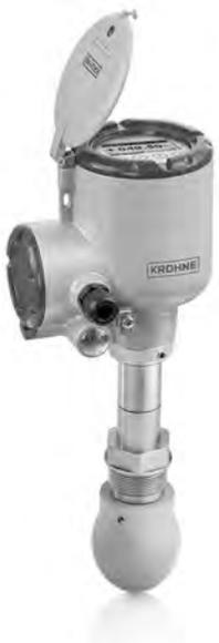
This 24 GHz FMCW radar level transmitter is designed for liquids in harsh environment like tanks with agitators containing corrosives or in non-Ex applications with extremely high process temperatures, like molten salt in solar plants (+700°C / +1292°F). For toxic and dangerous products, the use of a Metaglas® second sealing barrier is recommended.
