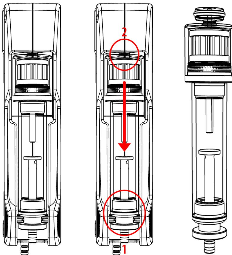
Remove the condensate separator by lifting it out from the groove (1) of the analyser. Then pull out the condensate separator downwards (2). Liquid discharged from the condensate separator may be slightly acidic. Condensate vessel and plug are screwed into each other. To change the pocket star filter and dry and clean the condensate separator, it can be easily disassembled and screwed back together.
