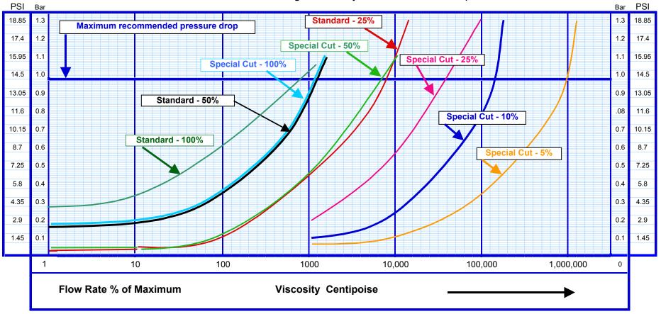
This graph is intended as an aid to determine the pressure drop of the measuring device as part of a system, allowing engineers to calculate the most economic components for their systems, i.e. pump selection would be determined on the total system pressure drop, the lower the pressure drop the lower the cost of the pumping component.
