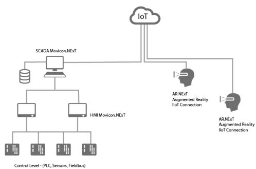
Example with Augmented Reality devices (for Hololens only) connected to systems via IIoT
