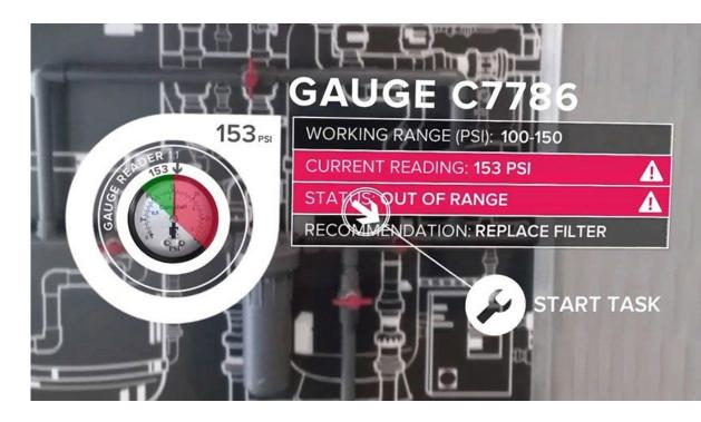
Example of Augmented Reality application where the display overlays dynamic data from the supervision system and the data server on the surrounding environment.
