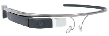
applications. This device offers several additional functions thanks to the integration of camera, inertia sensors, speakers and microphone, used for controlling Google Glass via vocal commands. It constitutes a real standalone wearable device, in that the application can be displayed directly on the glass and does not need any other external device. The product is still being tested, as Google is making hardware changes based on the user feedback.
