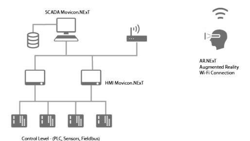
Example with Augmented Reality devices (Smartglass or Hololens) connected to systems via Wi-Fi network
