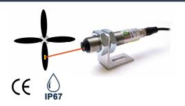
**RLS** (Rugged Laser Sensor): Threaded 316L stainless steel remote optical laser sensor with a visible red laser light source and green LED 'On Target' indicator. Performs over a wide speed range and operating envelope. The Rugged Laser Sensor is IP67 rated and includes a removable cable with water tight M12 connector for easy removal and cleaning.
