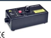
The *Smart Laser Sensor (SLS)* is an internal battery-powered optical speed sensor utilizing a visible Class 3R Laser for a TTL pulse output. Operating range up to 65 feet (19.8 m) with reflective tape and up to 3 feet (1 m) from contrasting color targets, keyways, bolt heads or blades.
