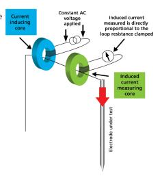
measurements. For the clamp-on method to work there must be a series-parallel resistance path (and the lower the better). The more electrodes or ground paths in the system the nearer the measurement gets to the actual electrode under test's true resistance. The following figure shows a pole ground configuration, one of the most effective applications of the clampon ground tester.
