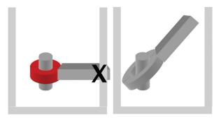
A larger inner area allows for clamping around larger ground rods or ground tapes (some of which can have a width of 50 mm). With a smaller internal opening on the instrument, the larger ground tape must be cut and a thinner copper bar welded in between to allow the instrument to make a measurement.
