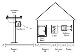
As most ground electrode testing takes place outside, users should consider buying an instrument rated to CATIV 600 V.
