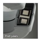
As mentioned in the section on potential sources of error on the previous page, dirt trapped between the closing gap in the clamp head can result in erroneous readings. Clamp-on ground testers are used outdoors in environments that are often dusty and dirty. They are exposed to materials that can end up on the core ends of the jaws. With flat core ends, the surfaces can be cleaned easily. This same material tends to get stuck in the interlocking teeth and is very hard to remove.
