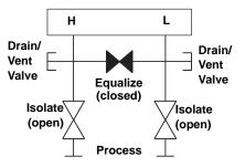
1. To zero the 3051, close the block valve to the low pressure (downstream) side of the transmitter first.
