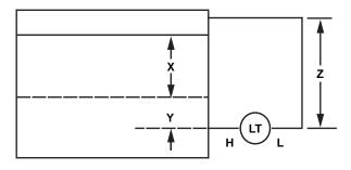
Let **X** equal the vertical distance between the minimum and maximum measurable levels (500 in.).
