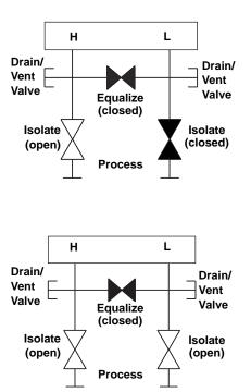
4. Open the block valve on the low pressure side of the transmitter to return the transmitter to service.
