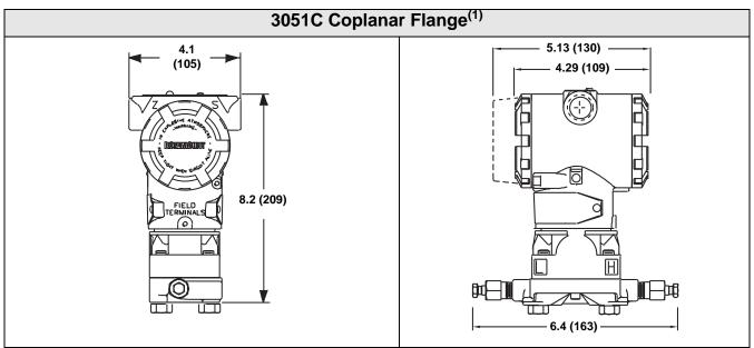
(1) For FOUNDATION fieldbus and Profibus PA transmitters with LCD Display, housing length is 5.36 in. (136 mm).
