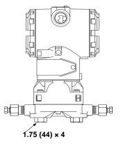
NOTE Dimensions are in inches (millimeters).
