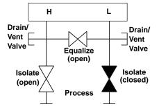
Open the center (equalize) valve to equalize the pressure on both sides of the transmitter. The manifold valves are now in the proper configuration for zeroing the transmitter. 3. After zeroing the transmitter, close the equalizing valve.
