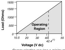
Communication requires a minimum loop resistance of 250 ohms. (1) For CSA approval, power supply must not exceed 42.4 V.
