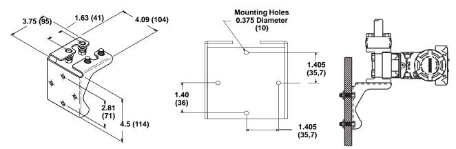
Figure 3-6. Flat Mounting Bracket Option Codes B3 and BC
